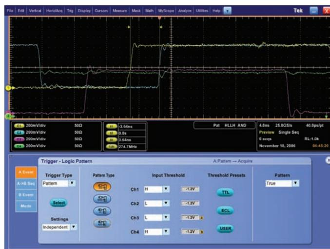
Figure 7a. Logic Pattern Triggering.
