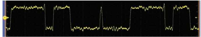
Figure 26. Glitch event detected using Pinpoint trigger type.
