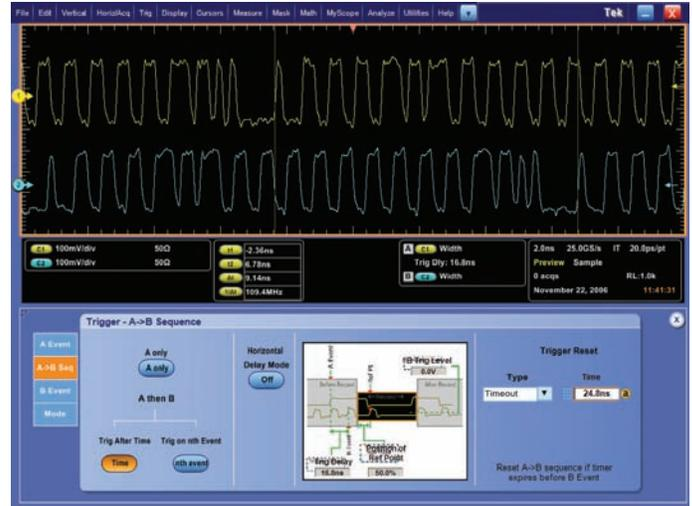
Figure 17. Serial Lane Violation Triggering.
