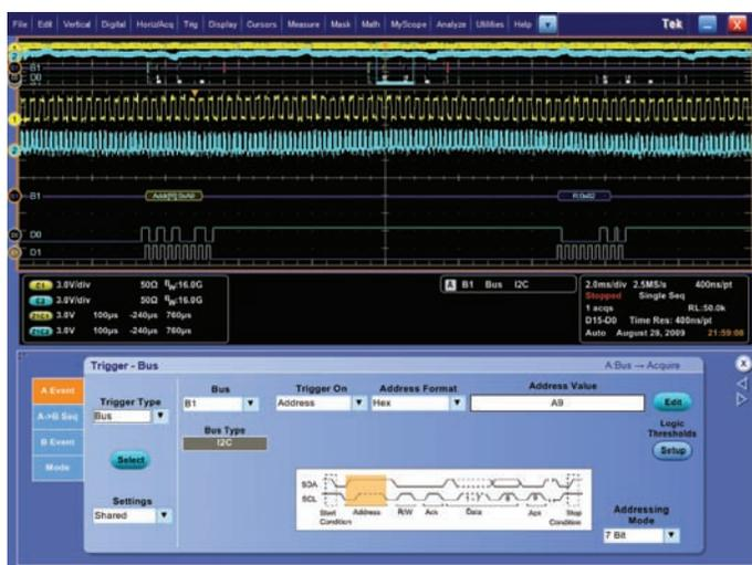
Figure 15. Low Speed Serial Protocol Triggering.
