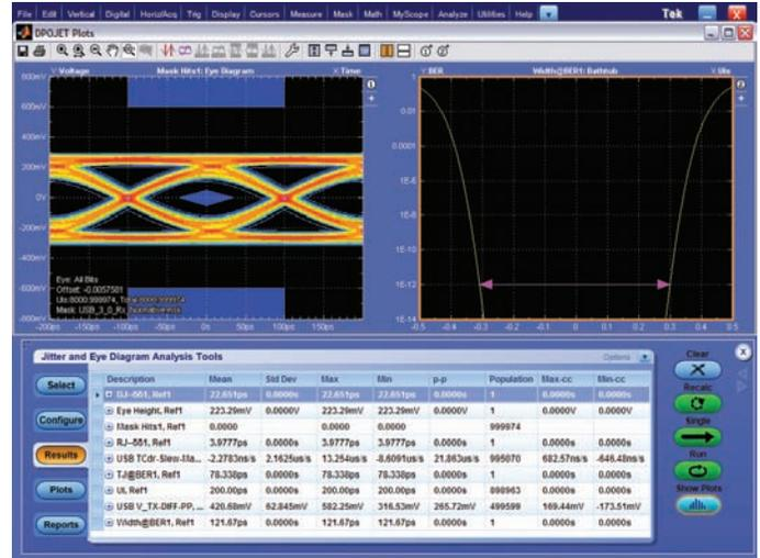
Figure 21. Lone Bit Pattern on DPOJET™.
