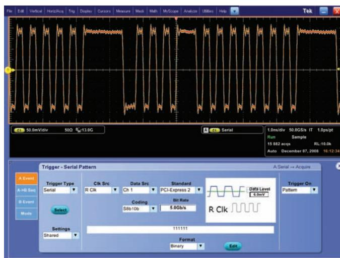
Figure 16. Serial Pattern Triggering.
