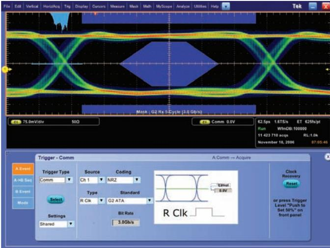
Figure 12. Communication Triggering.
