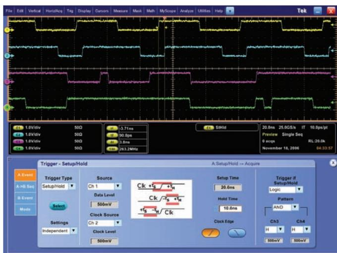
Figure 6. Logic Qualified Setup-and-Hold Triggering.
