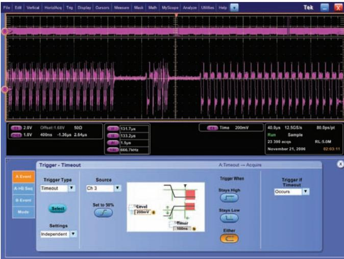
Figure 5d. Timeout Triggering.
