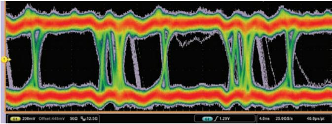
Figure 25. FastAcq visualization showing potential problems (in gray).
