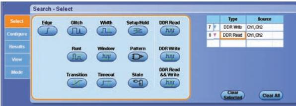
Figure 27. Pinpoint trigger type search methods.
