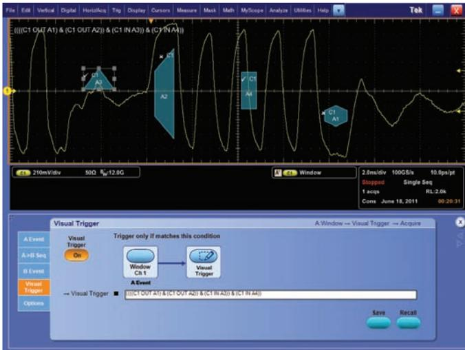
Figure 22. Visual Triggers on 70000 Series Oscilloscope.
