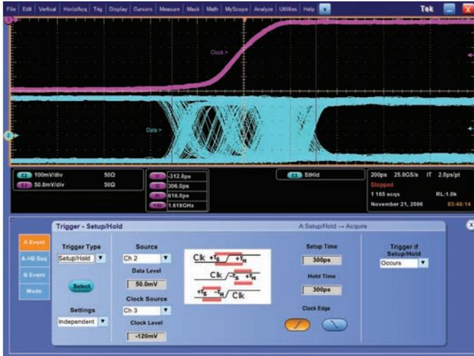
Figure 5f. Setup and Hold Triggering.
