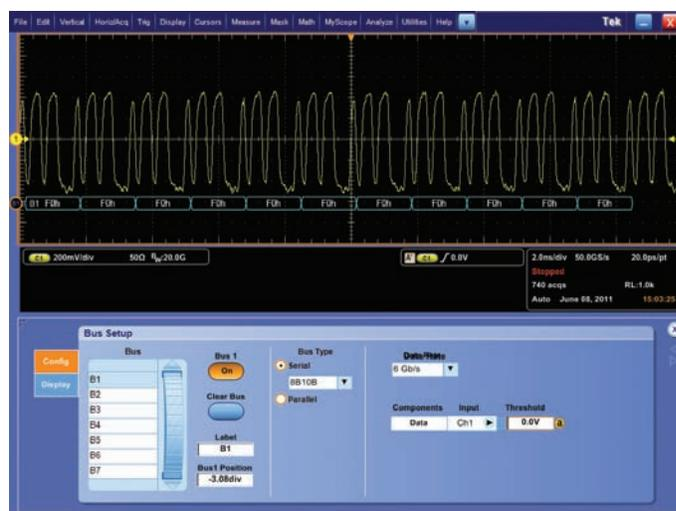
Figure 19. 8b/10b Serial Bus Trigger and Decode.
