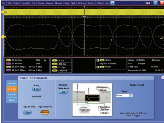
Figure 20. Lone Bit Pattern Trigger Setup.
