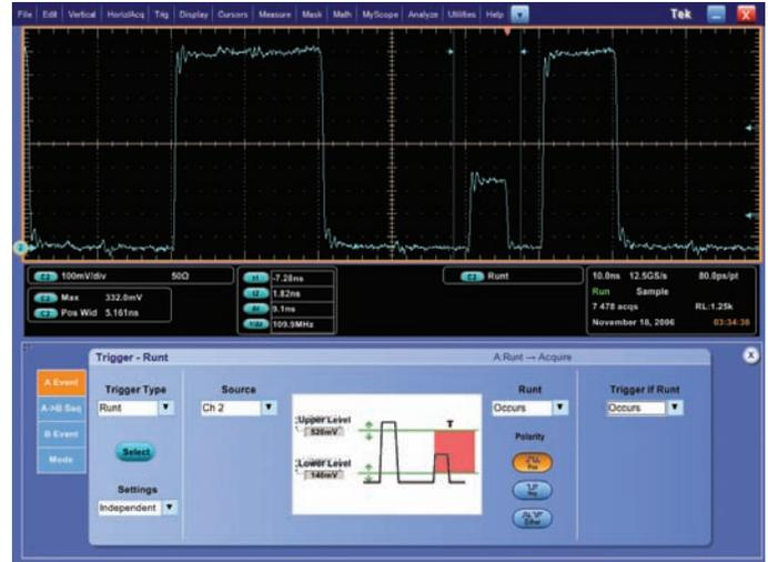
Figure 5c. Runt Triggering.
