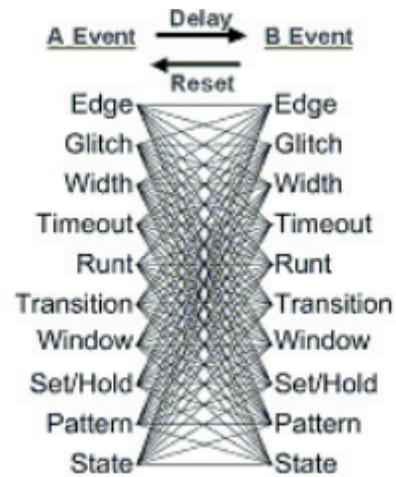
Figure 11b. Pinpoint Triggering - 1445 trigger combinations.
