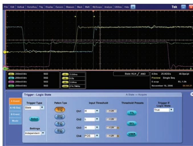
Figure 7b. Logic State Triggering.
