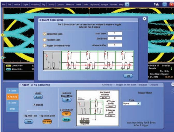
Figure 14. B-Event Scan Trigger Setup for DDR3.
