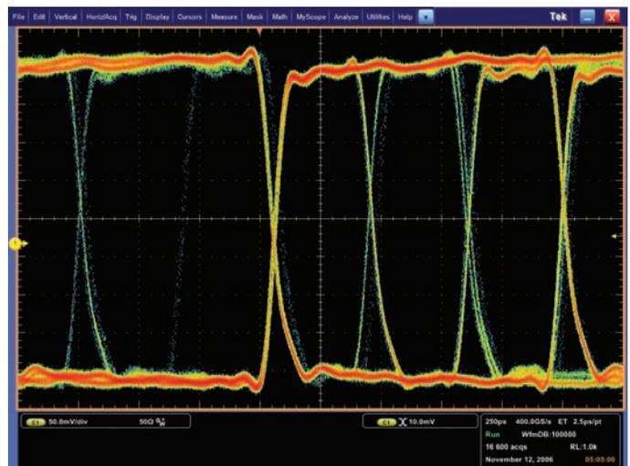
Figure 4c. Trigger Slope Positive and Negative.
