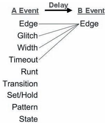
Figure 11a. Previous Generation Triggering - 17 trigger combinations.
