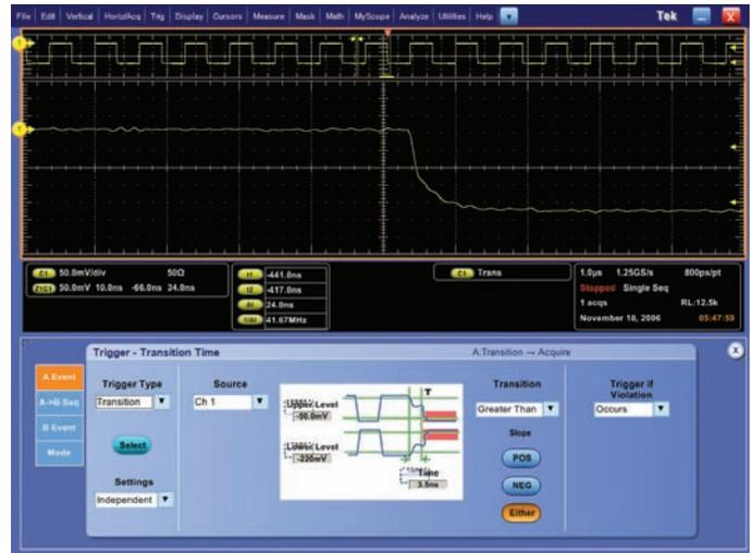
Figure 5e. Transition Time Triggering.
