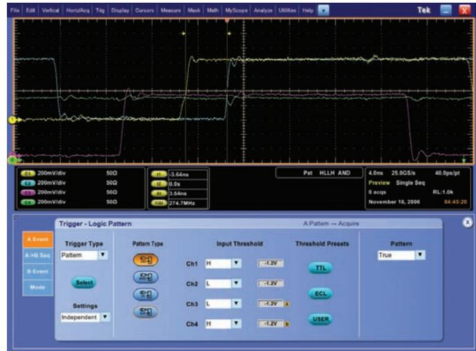
Figure 7a. Logic Pattern Triggering.
