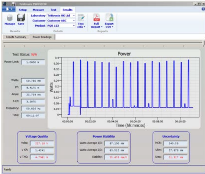
Figure 33. Tektronix PWRVIEW standby power measurement.
