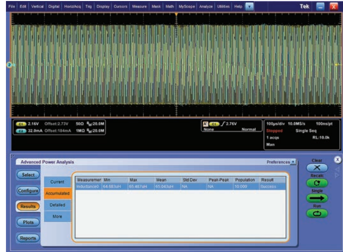
Figure 17. Inductance measurement results from DPOPWR application software.
