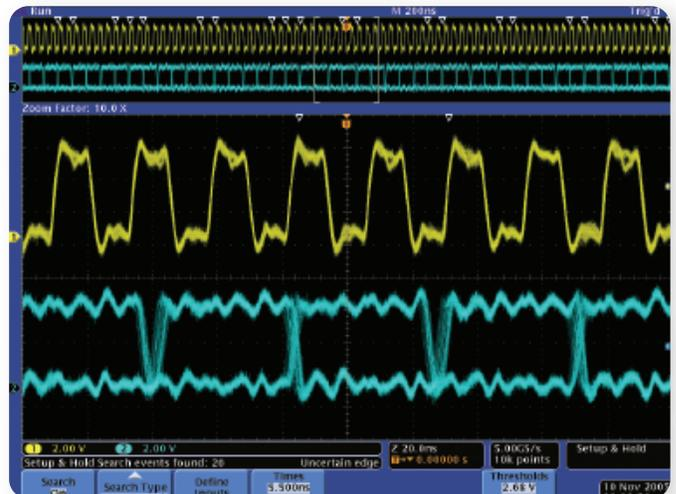
► **Figure 4.** The DPO4000 combines Search and Mark features with specialized Setup and Hold triggering. At the top of this display, the white hollow triangles mark all setup and hold violations with the user defined setup and hold times of 5.5ns and 4.5ns respectively.
