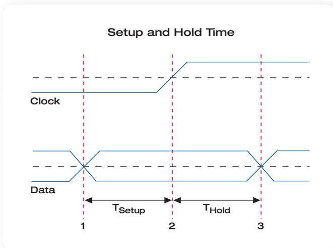
► **Diagram 2.** This diagram describes Setup time ( $T_{\text{setup}}$ ) and Hold time ( $T_{\text{hold}}$ ) definitions for a clocked logic circuit. Setup time is measured between points 1 and 2. Hold time is measured between points 2 and 3.
