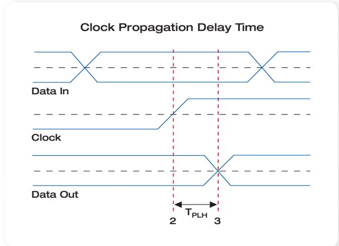
► **Diagram 3.** These signals illustrate the propagation time high-to-low ( $T_{PLH}$ ) and for a clocked logic circuit is measured between points 2 and 3.
