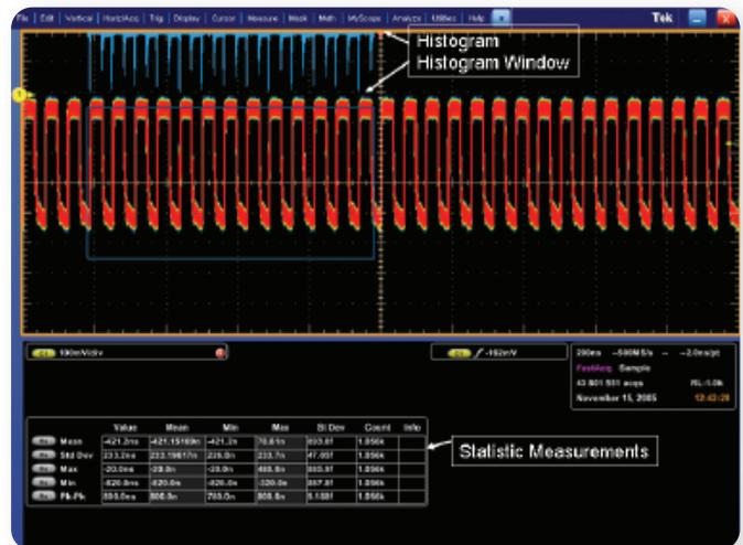
▶ **Figure 19.** The FastAcq acquisition mode on the DPO7000 with statistical measurements selected and displayed shows relatively stable clock signal on Ch 1. The histogram region is selected and turned on demonstrates how easily and rapidly design engineers can employ statistical analysis tools for confidence in compliancy.
