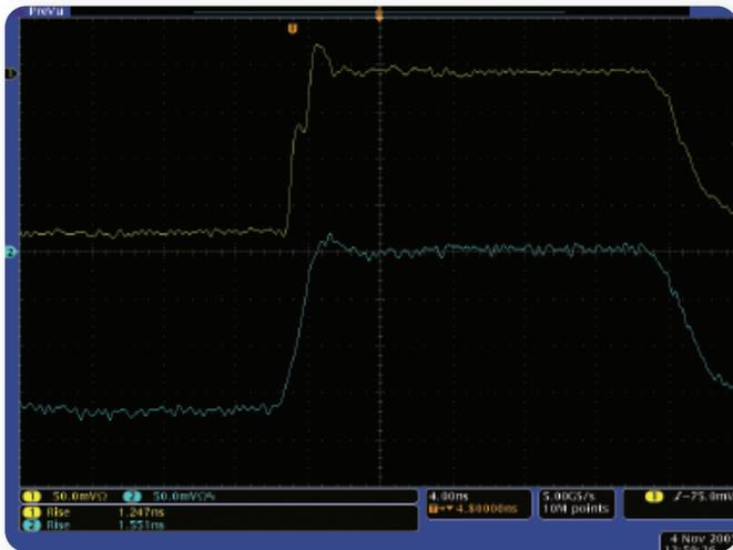
► **Figure 1.** The top signal (Ch 1) shows a 1.3 ns rising edge captured with a 1 GHz DPO4000. The bottom signal (Ch 2), is identical to the top but its bandwidth limited to 250 MHz showing what a 250 MHz oscilloscope might display. The reflection in the signal is masked by the insufficient bandwidth. (Note how insufficient bandwidth produces inaccuracies in signal rise time.)
