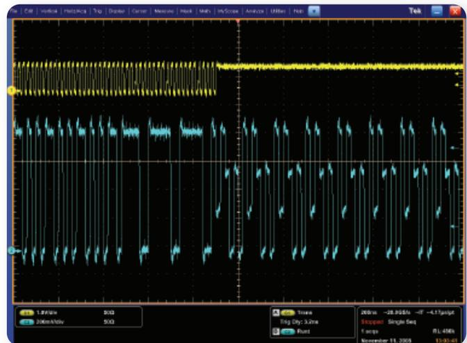
► **Figure 13.** The DPO7000 Pinpoint™ trigger makes it possible to use sophisticated trigger types for the B event as well as the A event. Here a B event is defined like A to isolate one bad transition followed by another. No matter if the B event arrives soon after an A event or much later. Either causes an acquisition. Runt logic pulses never cross through all the threshold levels necessary to become valid.
