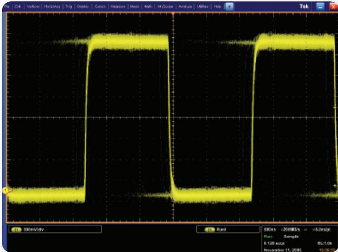
► **Figure 11.** A digital oscilloscope can show signals like they really are letting designers see how glitches affect design. Above the DPO7000 display shows very intermittent signal glitches using persistence. A persistence display generates a visual trace history.
