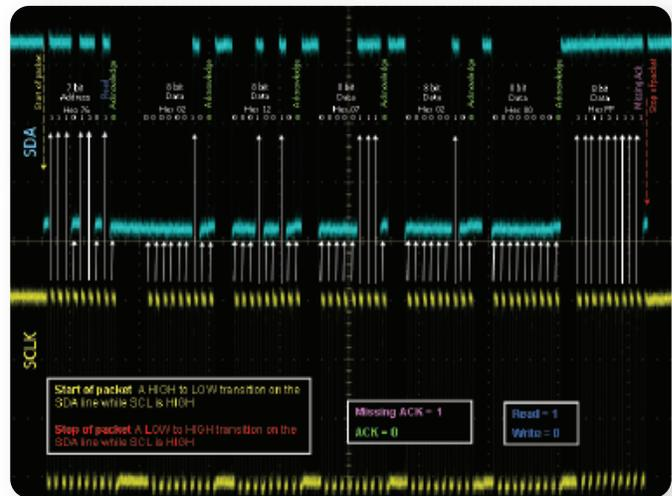
► **Figure 7.** A DPO display shows I<sup>2</sup>C Bus hand decoding. The address is 76, the operation is a read.
