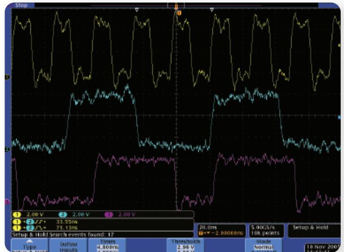
► **Figure 10.** Using the DPO4000 Setup and Hold Trigger and the Search/Mark capability show metastable states noted by the white triangles at the top of this display. Ch 1 is the clock signal and Ch 2 the data signal. Channel 3 is the metastable Q output of a D-type flip-flop latch.
