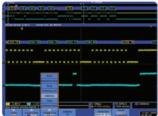
► **Figure 8.** The DPO4000 I<sup>2</sup>C Bus triggers on selected address 76 for a read or a write. Each packet is easily decoded eliminating hand decoding, reducing errors and saving time.
