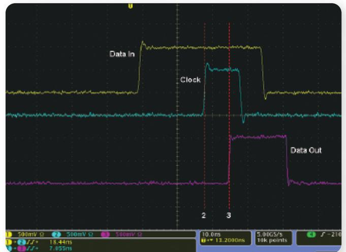
► **Figure 6.** The flexibility of the DPO4000 delay time measurement setup capability is used to measure clocked propagation delay time—this is the time measured between Data Out rising edge (point 3) with respect to the Clock rising (point 2). The clock propagation delay time is 7.055 ns.
