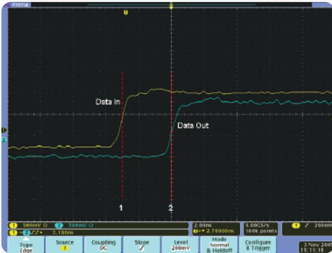
► **Figure 5.** The DPO4000 uses its delay time measurement capability to measure and display a propagation delay time, from Data In rising edge (point 1) to Data Out rising edge (point 2), to be 3.190ns.
