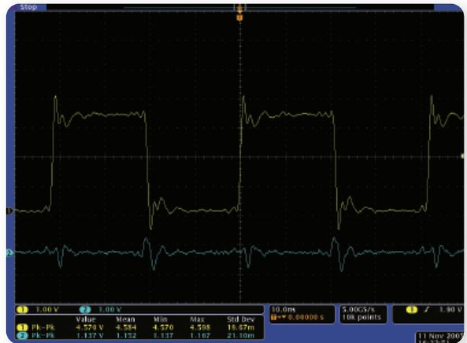
► **Figure 2.** Ground bounce from switching output on channel 1.
