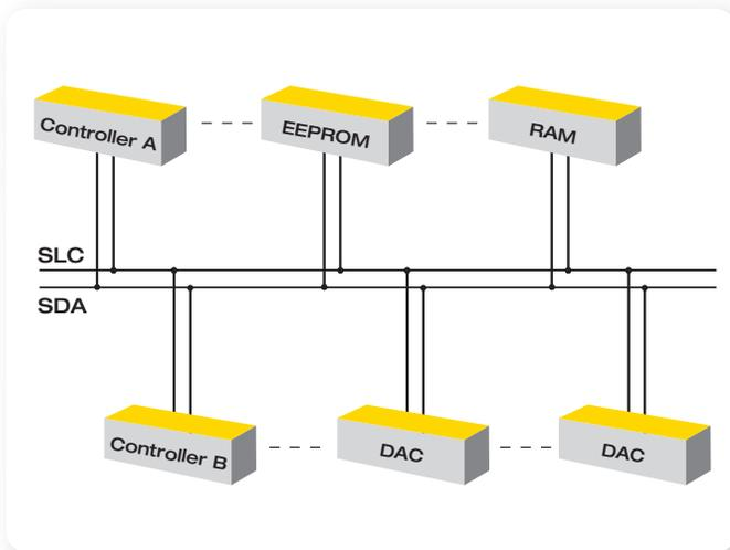
► **Diagram 4.** Diagram of I<sup>2</sup>C bus with various connected devices each selected by a unique address identifier contained in each serial packet transmitted.
