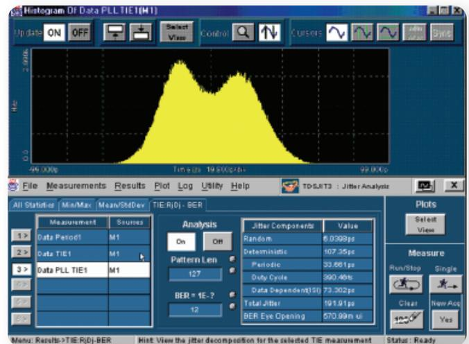
► **Figure 17.** DPO7000 with the TDSJIT3 Jitter Analysis application reveals a total jitter on the data signal equal to  $\sim 192$  ps ( $Tj = Dj + 2Q(BER) * Rj$ ), where  $Q(10E-12) = 7$ . The associated histogram of data PLL TIE measurement provides an engineer with a graphic representation of the data signals statistical distribution.
