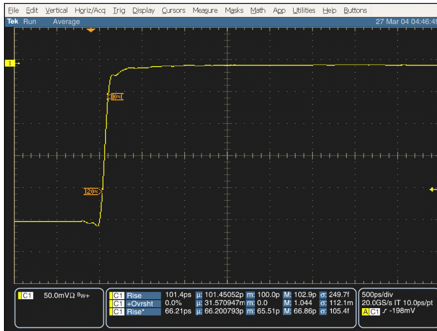
Figure 5. Tektronix TDS6804B oscilloscope gives 8 GHz bandwidth and measures the nominal 100 ps filter rise time as 101.4 ps.
