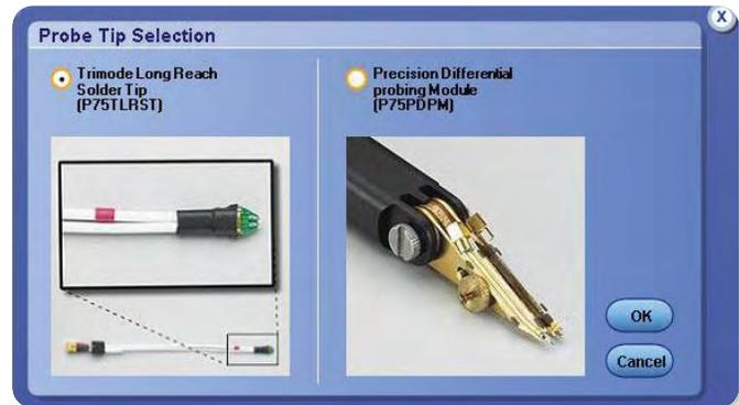
► **Figure 2.** P7500 Series Probe tip selection menu.
