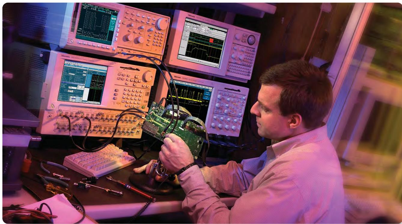
Real-time (RT) oscilloscopes have employed DSP (digital serial processing) filters to optimize magnitude and phase response and extend bandwidth beyond the analog -3 db bandwidth for several years. These same techniques are now extended to the oscilloscope probe tip. The resulting system response yields improved signal fidelity and often lower noise.
