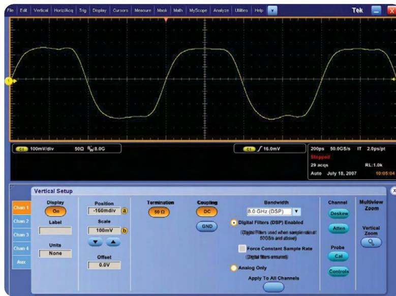
► **Figure 11.** 2.5 Gb/s PCI Express signal and Tektronix P7380 Medium Flex Small Resistor Tip-Clip with 8 GHz BWE DSP filter.
