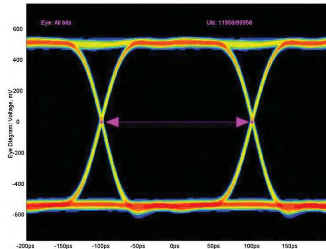
► **Figure 5.** P7516/P75LRST 5 Gb eye diagram with 16 GHz BWEH DSP filter.
