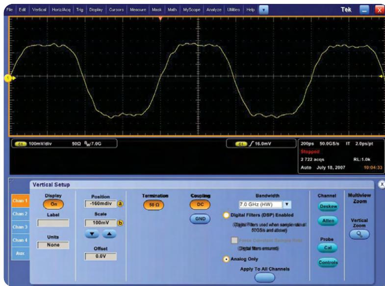
► **Figure 10.** 2.5 Gb/s PCI Express signal and Tektronix P7380 Medium Flex Small Resistor Tip-Clip without DSP filter.
