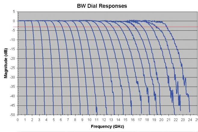
► **Figure 1.** Typical bandwidth limit filter response for the DPO/DSA70000 oscilloscopes.
