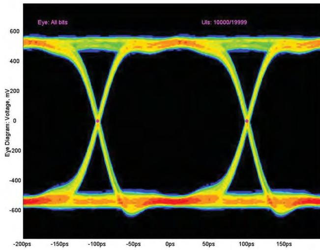
► **Figure 7.** P7516/7P5PDPM 5 Gb eye diagram without DSP filter.
