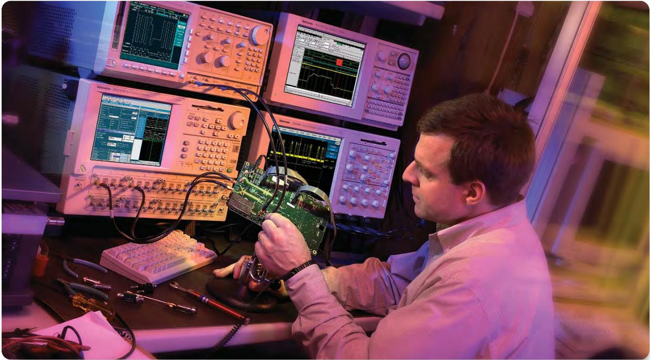
Real-time (RT) oscilloscopes have employed DSP (digital signal processing) filters to optimize magnitude and phase response and extend bandwidth beyond the analog -3 db bandwidth for several years. These same techniques are now extended to the oscilloscope probe tip. The resulting system response yields improved signal fidelity and often lower noise.
