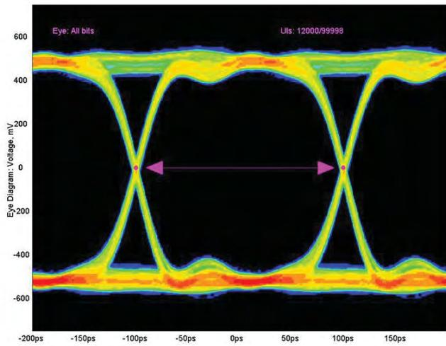
► **Figure 4.** P7516/P75LRST 5 Gb eye diagram without DSP filter.
