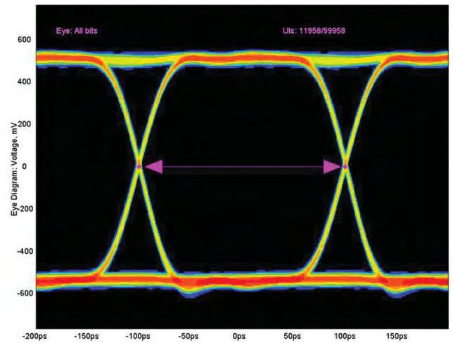
► **Figure 5.** P7516/P75LRST 5 Gb eye diagram with 16 GHz BWEH DSP filter.
