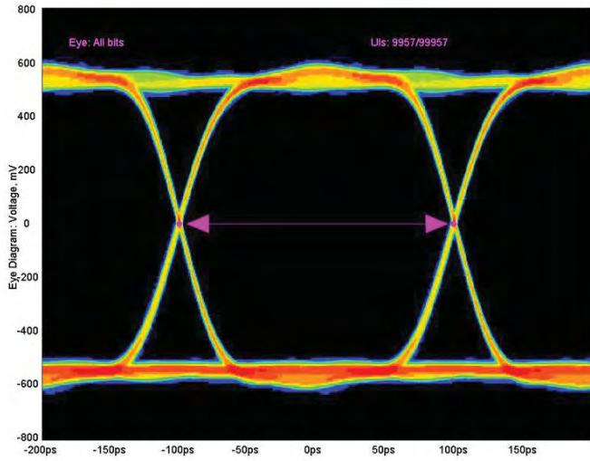
► **Figure 8.** P7516/7P5PDPM 5 Gb eye diagram with 16 GHz BWEEh DSP filter.
