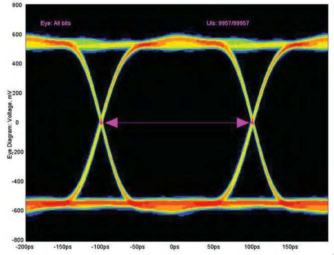
► **Figure 8.** P7516/7P5PDPM 5 Gb eye diagram with 16 GHz BWEh DSP filter.
