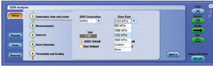
Figure 15. DDRA setup screen - Step 1.
