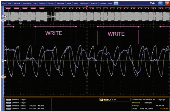
Figure 18. Back-to-back DDR3 Write operations.
