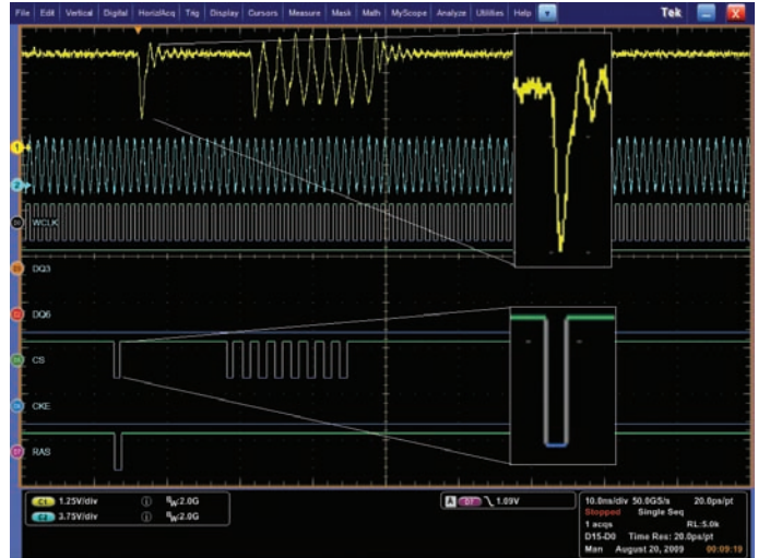
Figure 22. iCapture showing Chip Select line with analog and digital views.
