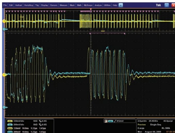
Figure 9. Using Advanced Search & Mark to identify all write bursts.
