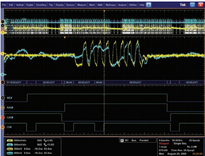
Figure 12. DDR3 Command Bus decoding on MSO70000.
