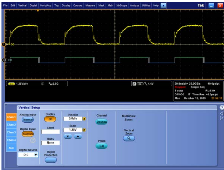
Figure 6. Edge ringing causing digital transitions.
