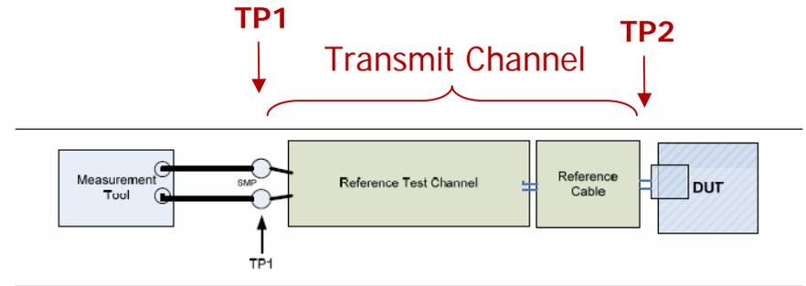
Figure 6-14. Tx Normative Setup with Reference Channel
