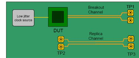
Figure 4-64: Tx Test Board Example
