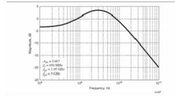
Figure 6-17. Tx Compliance Rx EQ Transfer Function
