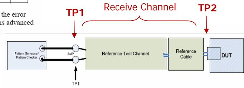
Source: USB 3.0 Specification Figure 6-18. Rx Tolerance Setup
