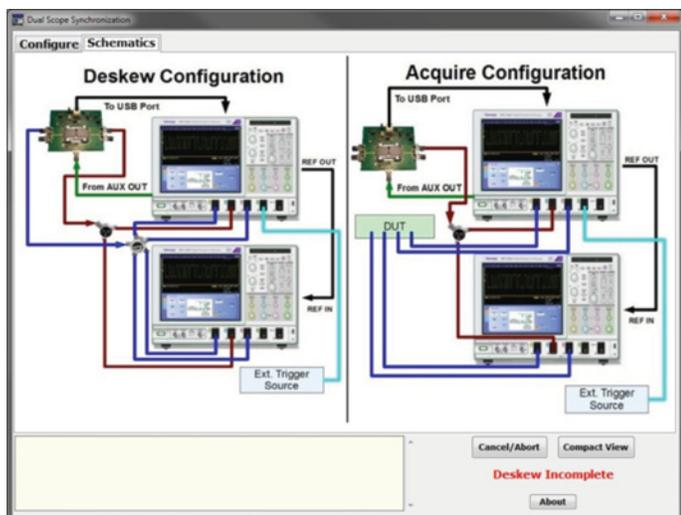
Figure 4. Schematic Tab, showing instrument connections for Deskew and Acquire operations.
