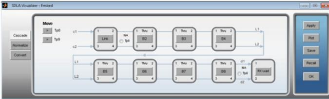
Figure 8. An example of a cascade of 4-port S-parameter blocks for modeling the simulated link model.
