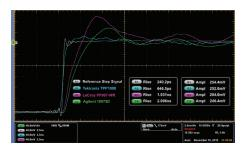
Comparison of a 0.2 ns edge observed with a Tektronix TPP1000 (blue), Keysight 10073D (green) and LeCroy PP007-WR (red)
