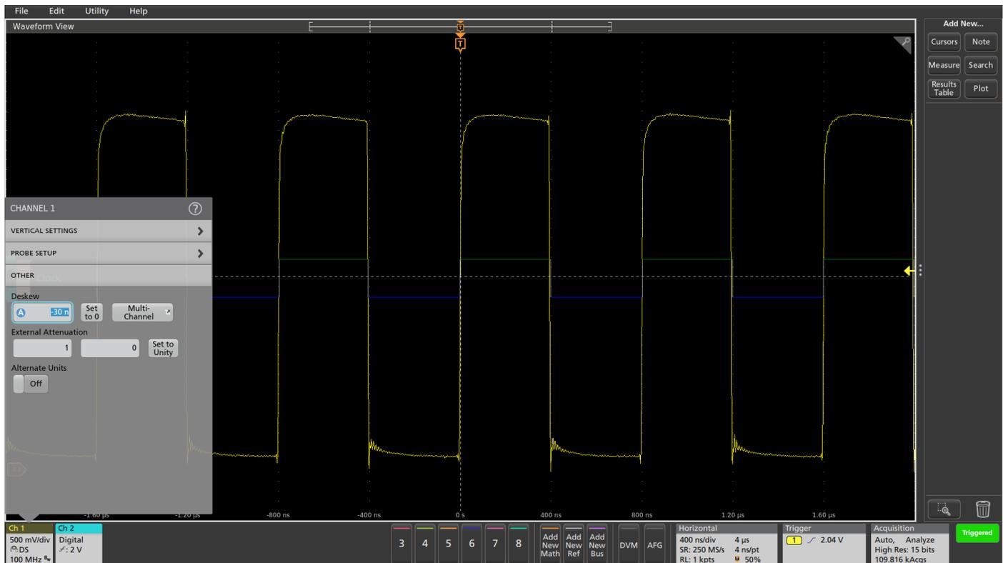
FIGURE 5. Analog channel time aligned with the digital channel.
