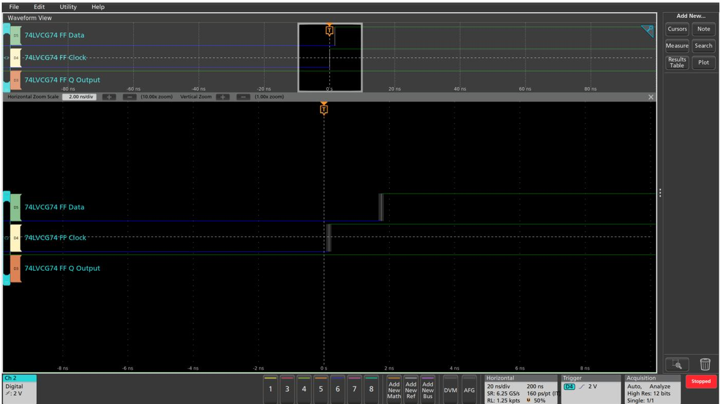
FIGURE 9. Hold time violation on a 74HCT74 flip-flop results in no change in Q output.
