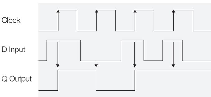
FIGURE 6. Example of flip-flop behavior.
