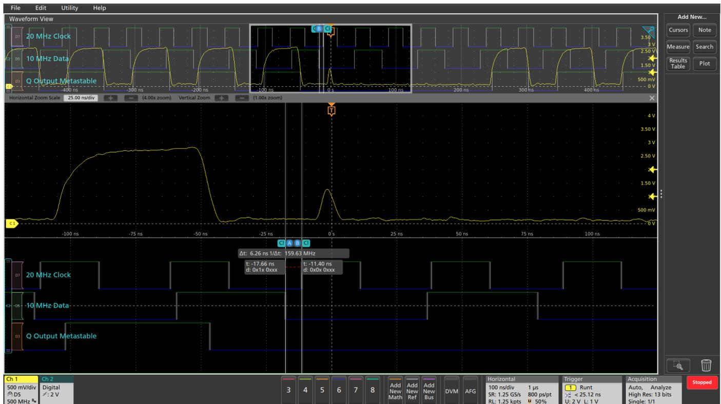
FIGURE 13. Cursor measurement of Setup Time violation triggering on a 74LVCG74 flip-flop.
