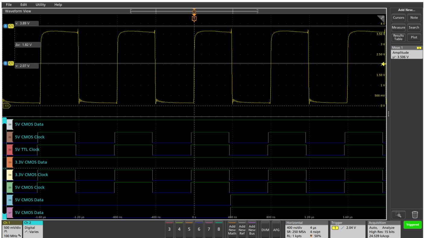
FIGURE 3. Probe color coding matches waveform color coding, making it easier to see which signals corresponds to which test point.
