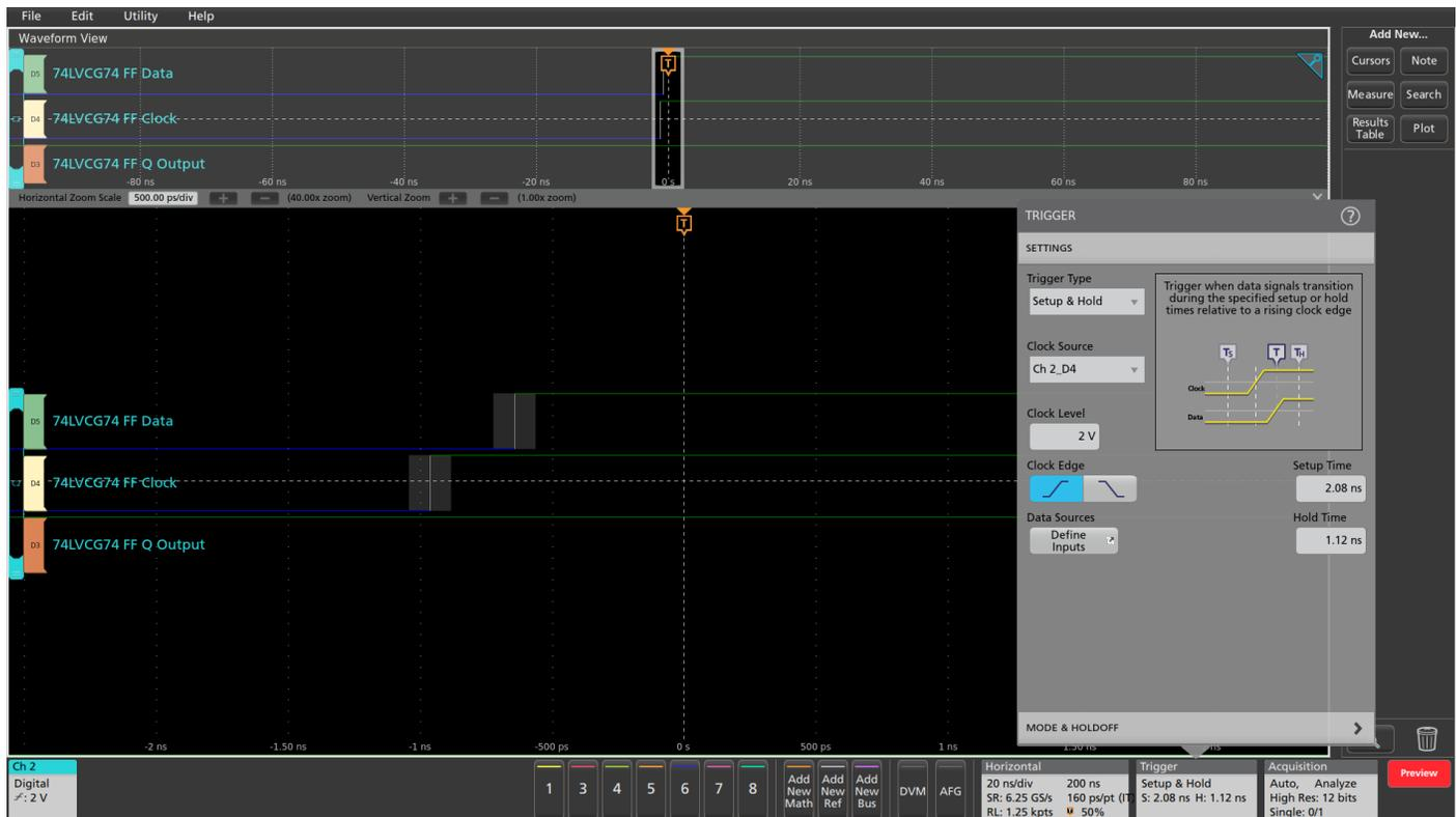
FIGURE 10. Automatic Setup and Hold violation triggering on a 74LVCG74 flip-flop captures many errors.
