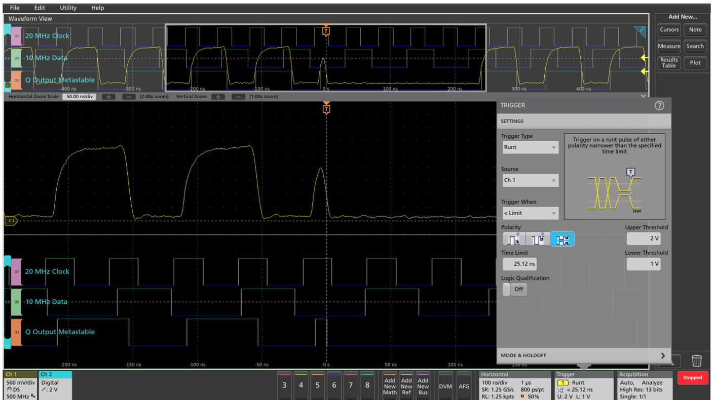
FIGURE 12. Runt triggering easily captures a low-amplitude, narrow pulse on the output of a 74LS74 flip-flop.
