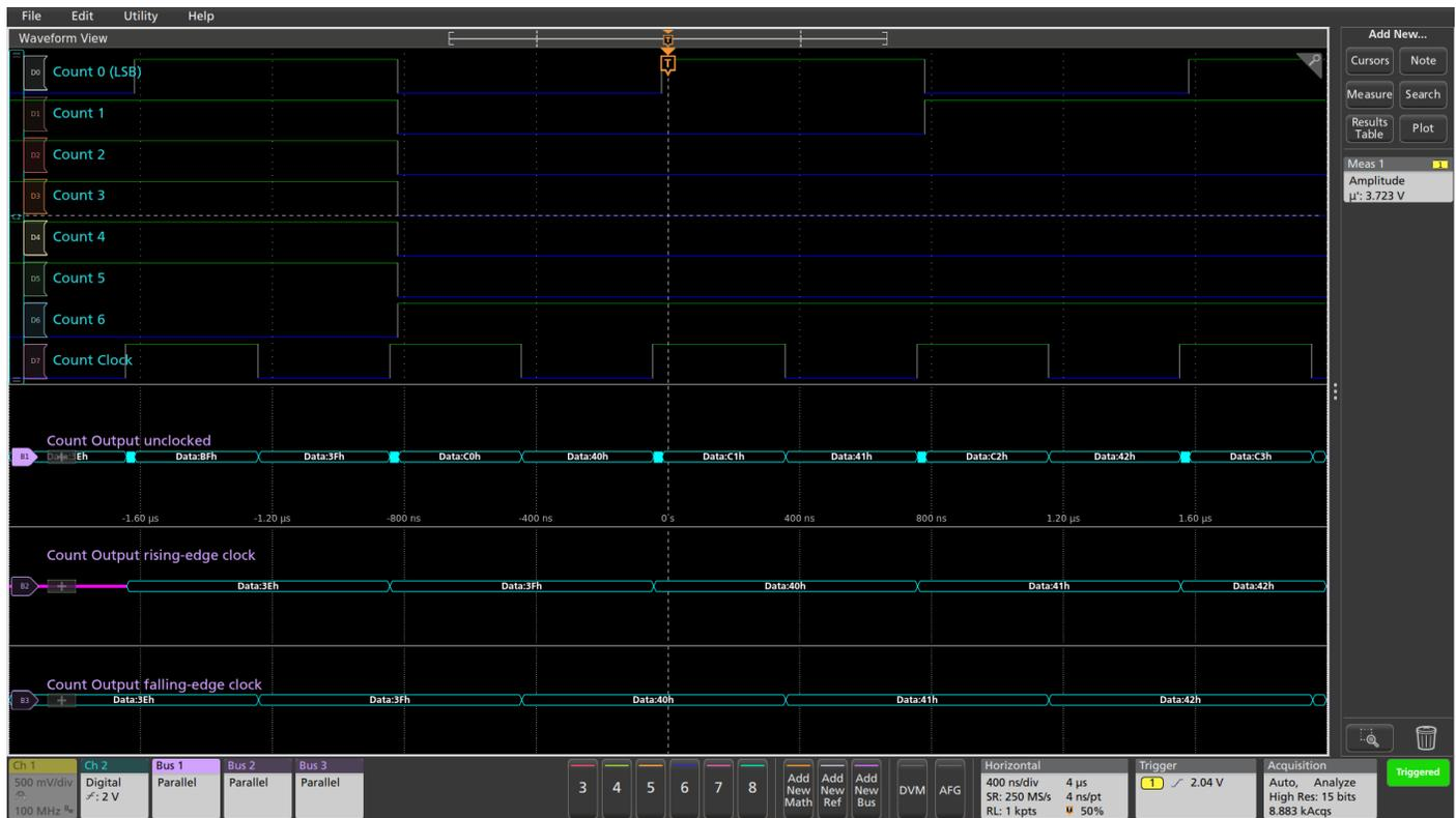
FIGURE 4. Example of a timing acquisition on the MDO/MSO Series. Three parallel buses have been defined and decoded using the device's clock signal.
