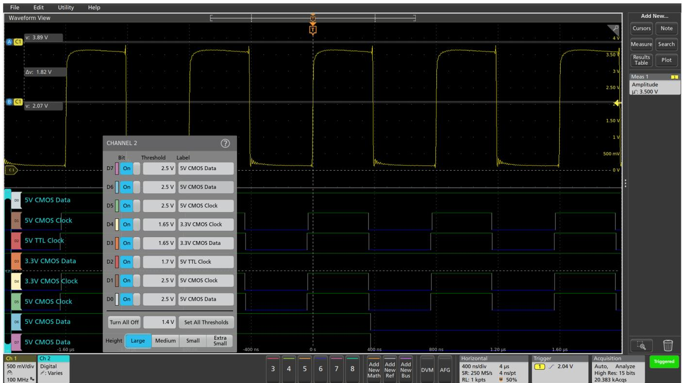
FIGURE 2. Mixed logic families (TTL & CMOS) threshold settings on the same TLP058 digital logic probe pod.
