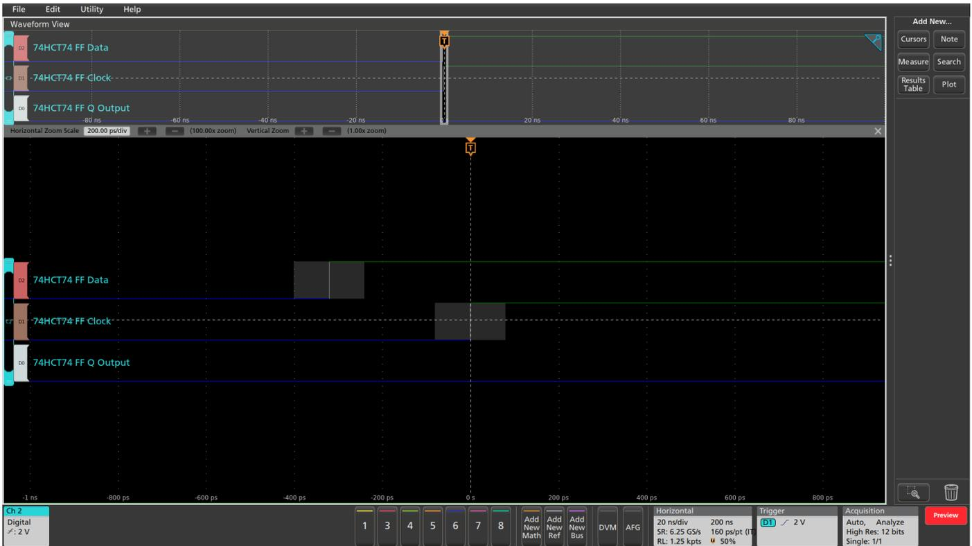
FIGURE 8. Setup time violation on a 74HCT74 flip-flop results in no change in Q output.
