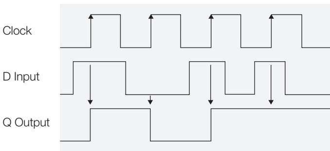
FIGURE 6. Example of flip-flop behavior.
