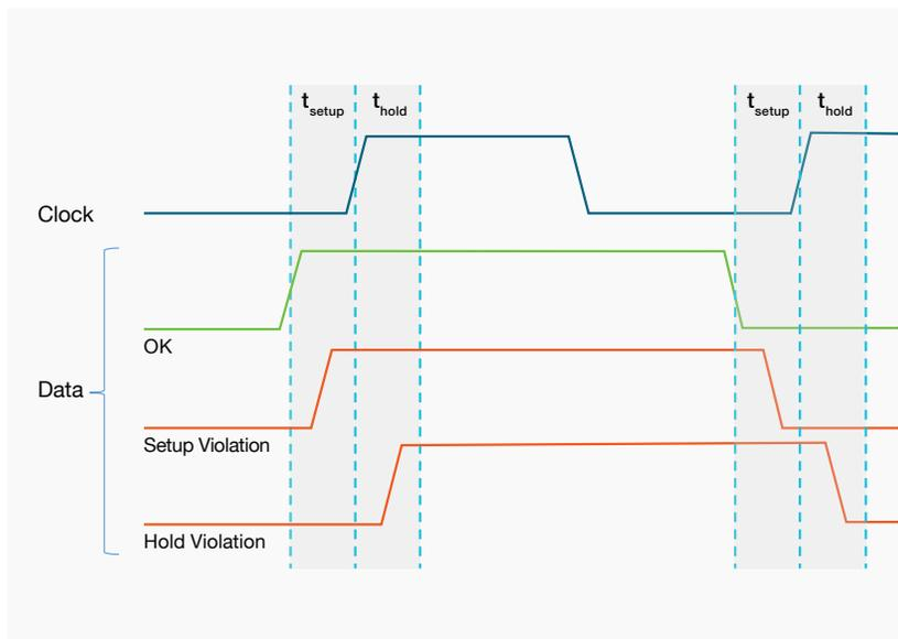
Setup Time is the time the input data signals are stable (either high or low) before the active clock edge occurs. Hold Time is the time the input data signals are stable (either high or low) after the active clock edge occurs. Setup and Hold Times are specified in component data sheets for synchronous devices (such as flip-flops) and must be met to assure that the component will behave correctly and reliably.
