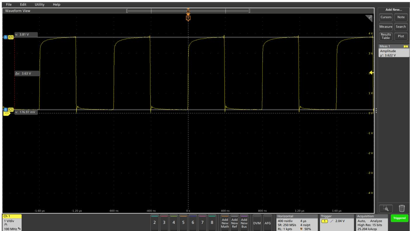
FIGURE 1. Quick verification of the logic signal amplitude using automated measurements.
