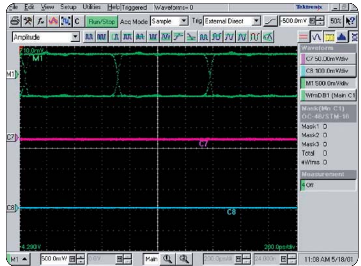
► Figure 3. 1.5 Gb/s signal with no probe loading.
