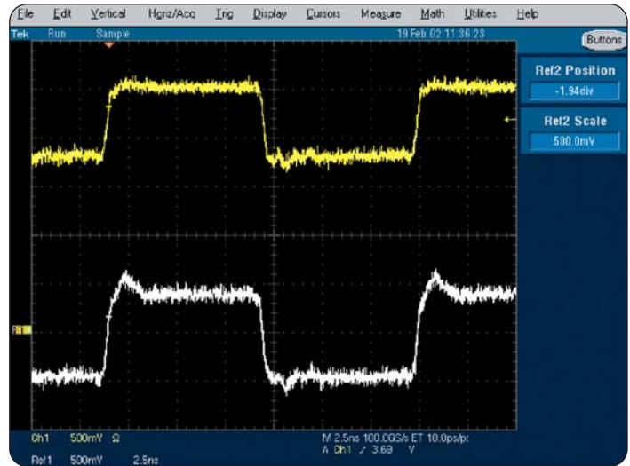
► Figure 2. Example of signal compression (top trace) caused by exceeding the dynamic range.
