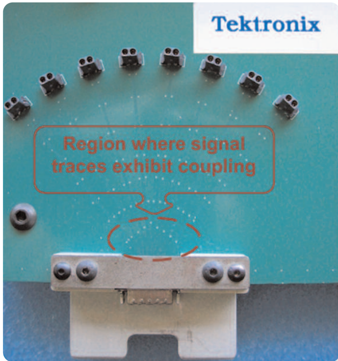
► Figure 2. Gore InfiniBand 4x test fixture. The differential traces become coupled at the high-speed connector receptacle area.
