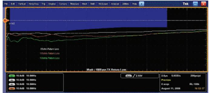
Figure 4.  $85/100/115 \Omega$  plots for the Return Loss measurement.
