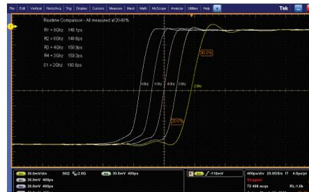
Figure 6. Risetime measurements at various bandwidths.
