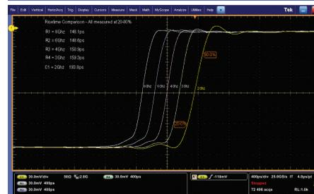
Figure 6. Risetime measurements at various bandwidths.
