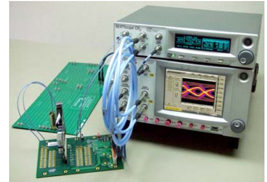
Stressed Receiver Tolerance Testing with a BERTScope
