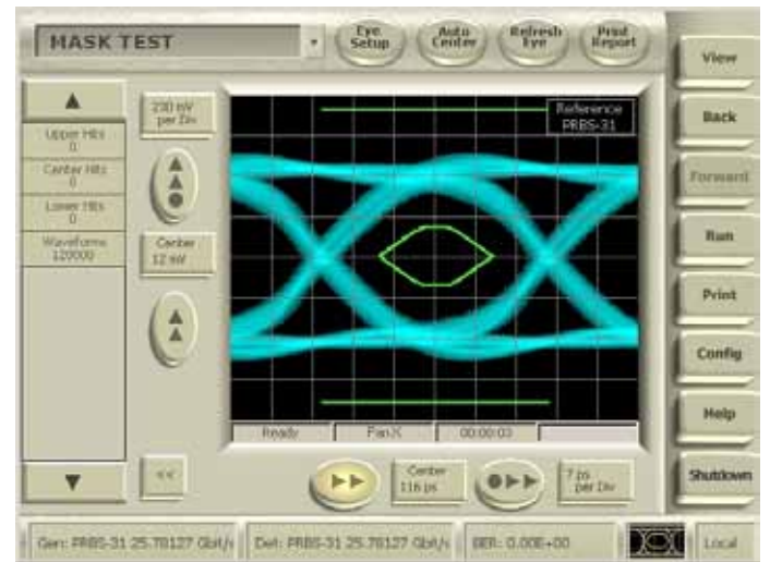
Figure 4b. 100GbE Eye Mask on a BERTScope.
