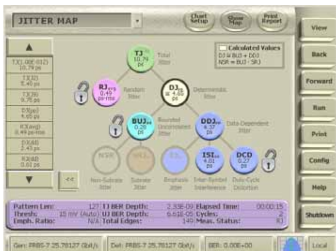
Figure 16. Example of jitter decomposition on a BERTScope.
