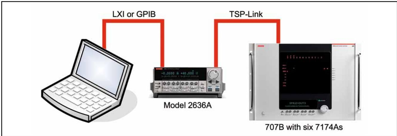
Series 2600A SMUs have an on-board test script processor (TSP) that executes test scripts and controls the switch matrix via the TSP-Link, which acts like a hardware backplane, connecting the two high-performance processors at full hardware speeds. This configuration provides the best possible throughput and flexibility and the tightest synchronization between the instrument and the switch matrix.
