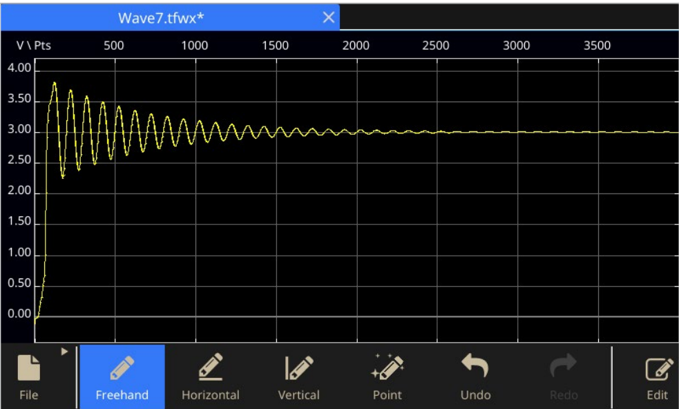
Figure 10: Freehand drawing to create transient response of RLC circuit in ArbBuilder.
