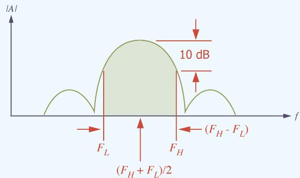
► **Figure 8.** US FCC defined a UWB signal as any signal with a bandwidth at the 10 dB attenuation points ( $> 90\%$  spectral power bandwidth) greater than 20% of the modulation frequency.
