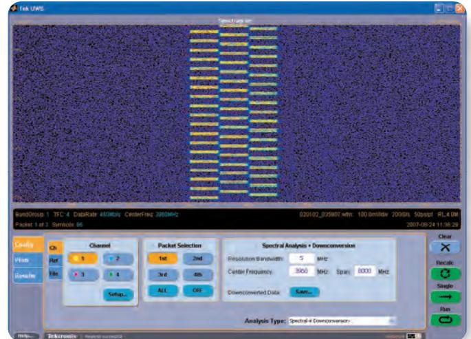
▶ **Figure 14.** A WiMedia MB-OFDM signal with frequency hop spreading is captured with a DPO7000 series oscilloscope and displayed as a spectrogram of the band group.
