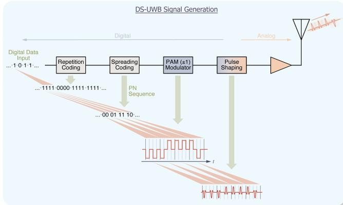
▶ **Figure 13.** DS-UWB PAM signal generation is similar to TH-UWB. A key difference is in the pulse modulator that inverts the phase of the pulse.
