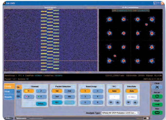
► **Figure 23.** UWB analysis software measures the constellation of a single OFDM carrier as well as EVM, data rate and center frequency.
