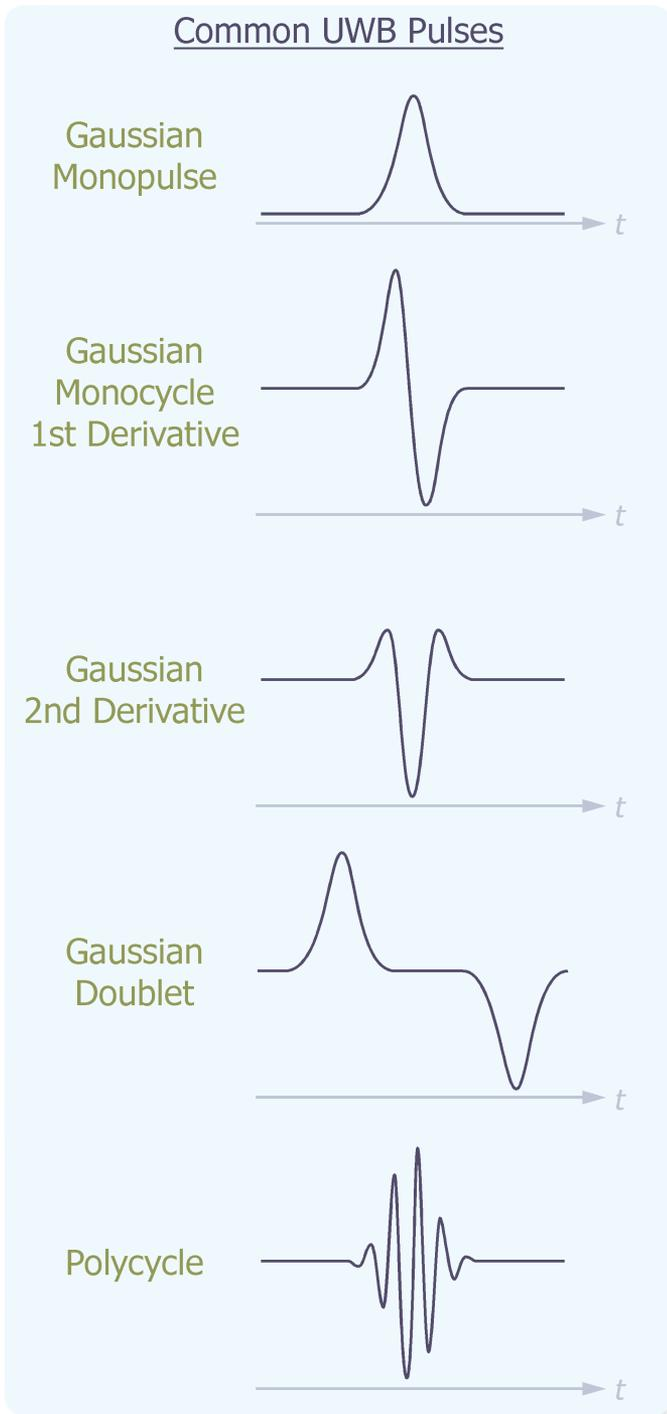
► **Figure 11.** A variety of Gaussian impulse shapes are commonly used with UWB signals. The simple Gaussian monopulse is shown for reference only, and is rarely used because it introduces a DC offset.
