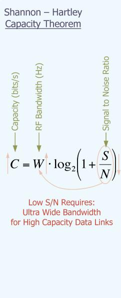
► **Figure 2.** The Shannon–Hartley theorem illustrates the ideal relationship between channel capacity ( $C$ ), RF bandwidth ( $W$ ) and minimum signal-to-noise ( $S/N$ ) ratio. UWB is attractive because high channel capacities or data rates can be supported with low  $S/N$  ratios. Comparing the RF bandwidth and  $S/N$  requirements for the illustrated modulations with identical bit rate capacity, it is easy to see bandwidth can be traded for  $S/N$  Ratio.
