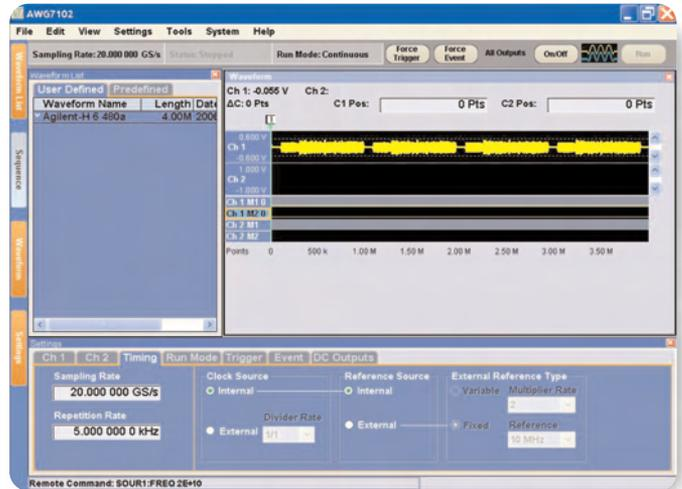
▶ **Figure 17.** The Tektronix AWG7000 arbitrary waveform generator can directly generate many UWB signals with its 20 GS/s capability.
