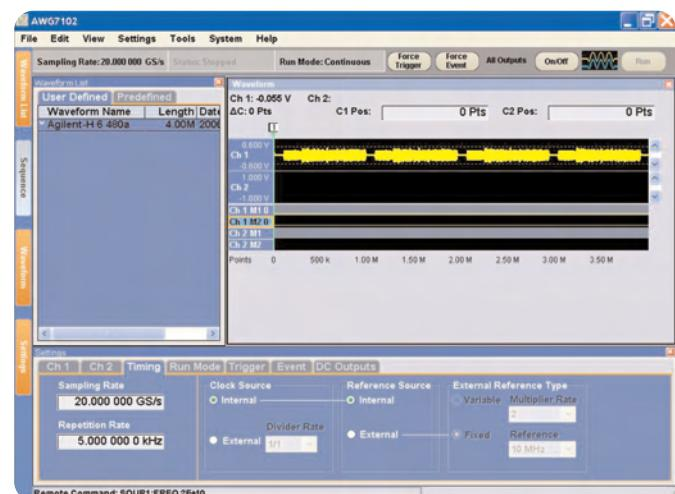
► **Figure 17.** The Tektronix AWG7000 arbitrary waveform generator can directly generate many UWB signals with its 20 GS/s capability.
