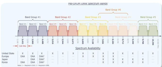
► **Figure 15.** The WiMedia band group structure provides several band groups for its MB-OFDM signal structure. Not all bands are available worldwide and some require a DAA for interference mitigation.
