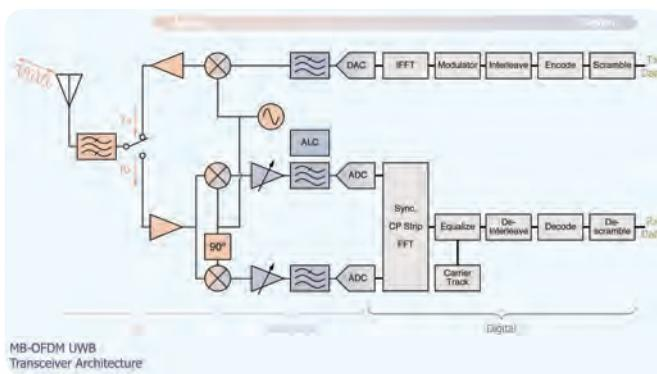
► **Figure 16.** The MB-OFDM transceiver architecture shows the benefits of a homodyne zero-IF design. The high levels of digital implementations eliminate many expensive IF and RF components.
