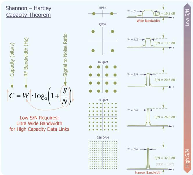
▶ **Figure 2.** The Shannon–Hartley theorem illustrates the ideal relationship between channel capacity ( $C$ ), RF bandwidth ( $W$ ) and minimum signal-to-noise ( $S/N$ ) ratio. UWB is attractive because high channel capacities or data rates can be supported with low  $S/N$  ratios. Comparing the RF bandwidth and  $S/N$  requirements for the illustrated modulations with identical bit rate capacity, it is easy to see bandwidth can be traded for  $S/N$  Ratio.
