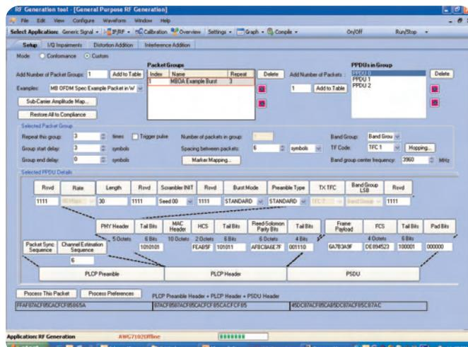
► **Figure 20.** RFXpress can synthesize WiMedia packet waveforms from the packet group level controlling PLCP preamble, header and PSDU data payload.
