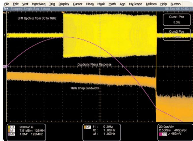
► **Figure 5.** A 1 GHz radar chirp is captured with the DPO7000 oscilloscope using its 20 GHz of bandwidth. The oscilloscope can convert the time domain signal (yellow) to a spectral plot (orange) and phase (purple).
