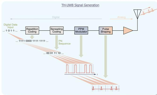
▶ **Figure 9.** TH-UWB generation with PPM is a simple process of coding, spreading, modulating and shaping the short impulses that make up the signal. Notice how the signal creation is all done at base-band with no frequency up-conversion.
