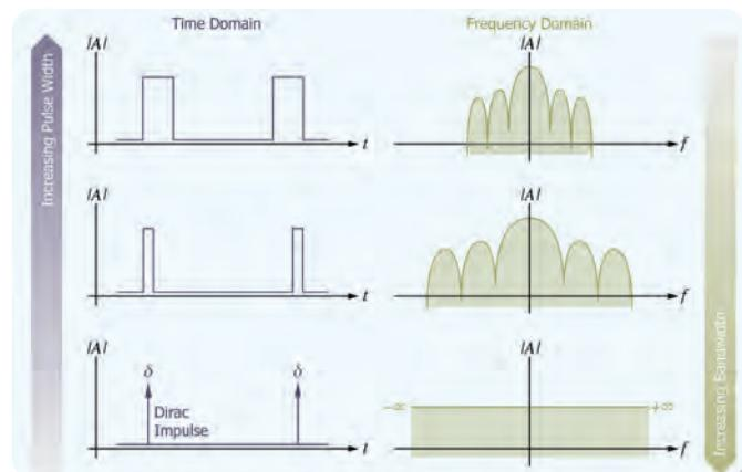
► **Figure 10.** Pulsed signal bandwidth is inversely related to pulse width in the time domain. Thus changing the time domain impulse shape can control the power spectral density of a UWB signal.
