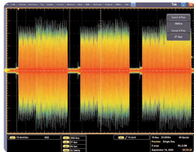
► **Figure 6.** Powerful UWB test instruments Like the AWG7000 series and DPO70000 can generate and capture complex ultra-wideband signals.
