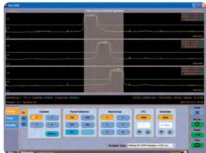
► **Figure 21.** The spectral mask for each band of the WiMedia band group along with the ACPR measurements are simultaneously tested on the DPO7000 series oscilloscope with UWB application software.
