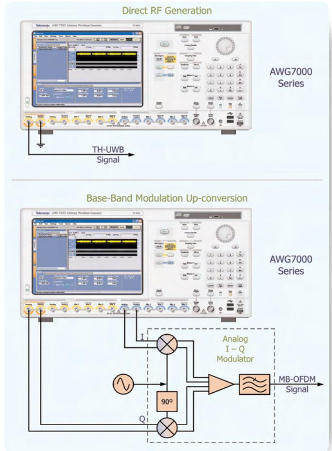
► **Figure 18.** AWG7000 supports direct base-band and external I-Q modulator/up-converter UWB signal generation approaches.
