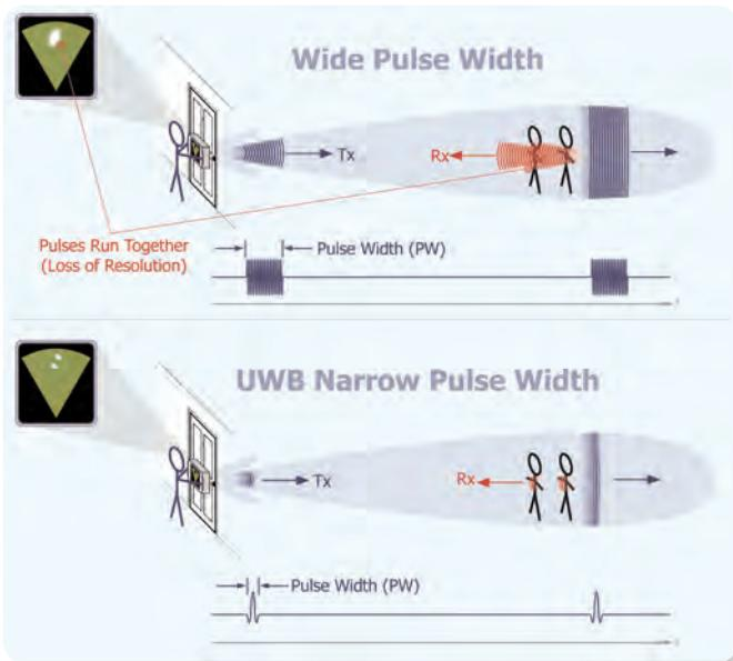
► **Figure 4.** Longer radar pulse widths can run together, being interpreted as a single echo return or object. Short UWB pulse-widths improve the radar's resolution by returning distinctly separate echoes.
