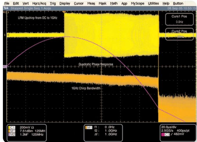
► **Figure 5.** A 1 GHz radar chirp is captured with the DPO7000 oscilloscope using its 20 GHz of bandwidth. The oscilloscope can convert the time domain signal (yellow) to a spectral plot (orange) and phase (purple).
