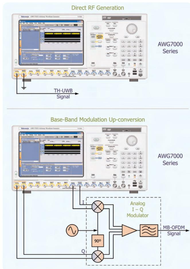
► **Figure 18.** AWG7000 supports direct base-band and external I-Q modulator/upconverter UWB signal generation approaches.
