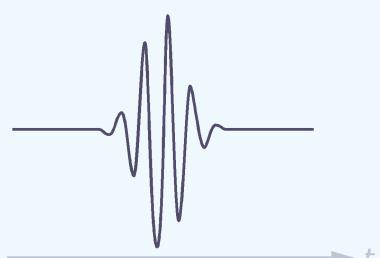
► **Figure 11.** A variety of Gaussian impulse shapes are commonly used with UWB signals. The simple Gaussian monopulse is shown for reference only, and is rarely used because it introduces a DC offset.
