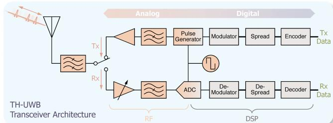
► **Figure 12.** TH-UWB transceiver architectures can be very simple and lack many traditional analog RF components. TH-UWB signals can be created and processed almost entirely at base-band with digital hardware.
