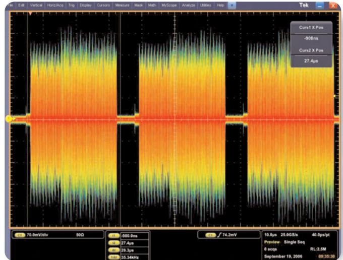
► **Figure 6.** Powerful UWB test instruments like the AWG7000 series and DPO70000 can generate and capture complex ultra-wideband signals.
