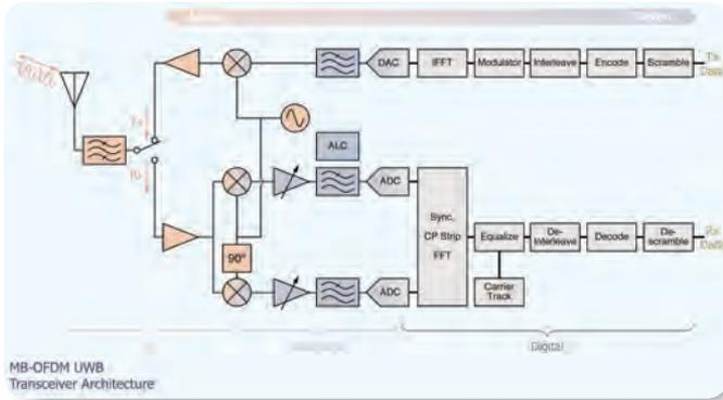
▶ **Figure 16.** The MB-OFDM transceiver architecture shows the benefits of a homodyne zero-IF design. The high levels of digital implementations eliminate many expensive IF and RF components.
