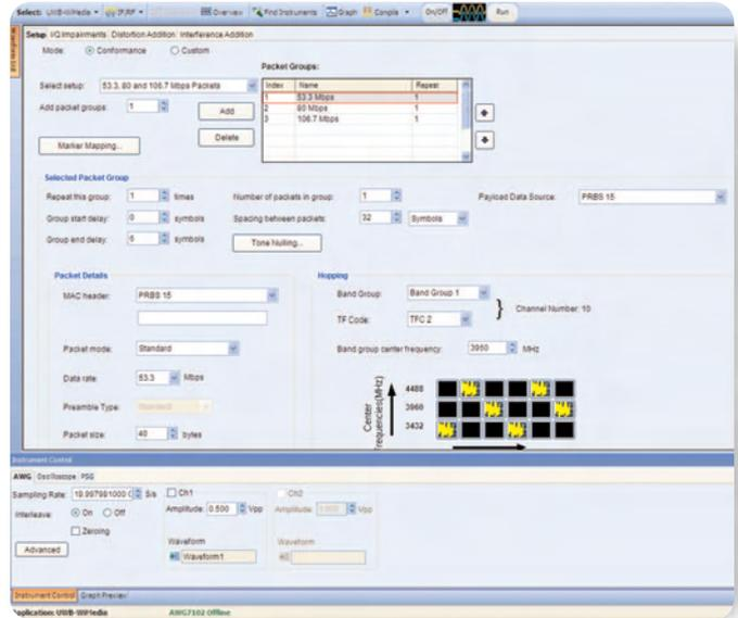
▶ **Figure 19.** RFXpress offers both general purpose multi-channel modulation synthesis and standards based synthesis like WiMedia’s UWB signals.
