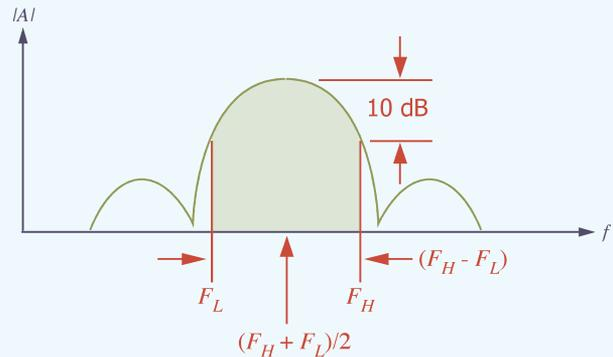
► **Figure 8.** US FCC defined a UWB signal as any signal with a bandwidth at the 10 dB attenuation points (? 90% spectral power bandwidth) greater than 20% of the modulation frequency.
