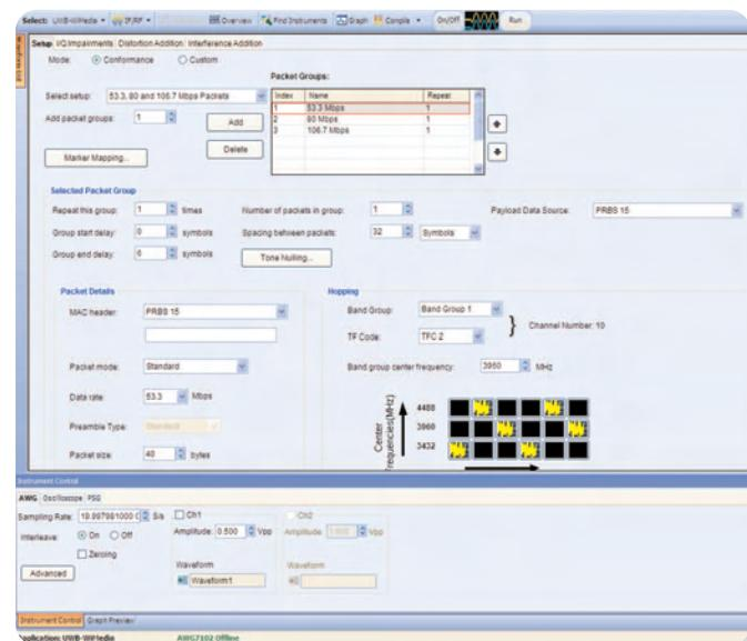
► **Figure 19.** RFXpress offers both general purpose multi-channel modulation synthesis and standards based synthesis like WiMedia’s UWB signals.
