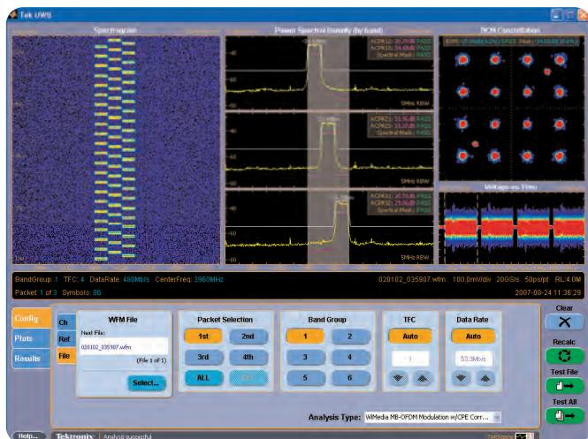
► **Figure 22.** The DPO7000 oscilloscope and UWB analysis software automatically identifies the TFC of this MB-OFDM spectrogram as part of a complete set of measurements and plots for each analyzed packet.
