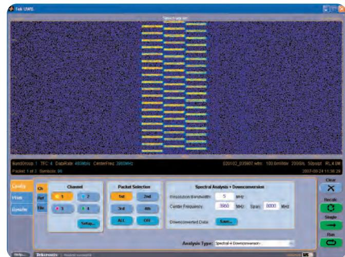
► **Figure 14.** A WiMedia MB-OFDM signal with frequency hop spreading is captured with a DPO7000 series oscilloscope and displayed as a spectrogram of the band group.
