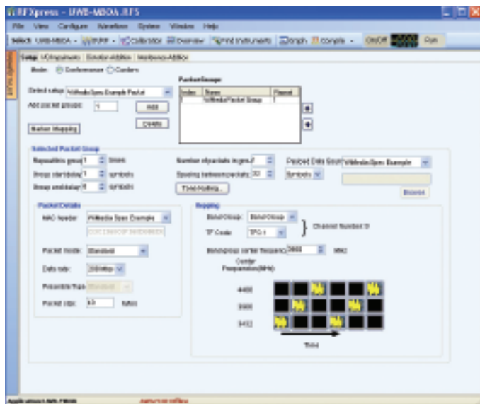
Figure 7. UWB-WiMedia signal generation in RFXpress conformance mode.
