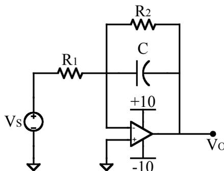
**Figure 7. An Active Low Pass Filter.**
