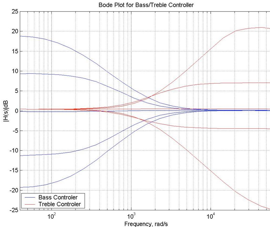
**Figure 14. Example Bode Plots from Active Tone Controller.**
