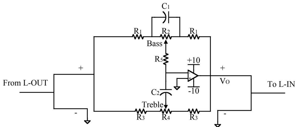
**Figure 15. Input and Output Connectinos to Tone Controller.**
