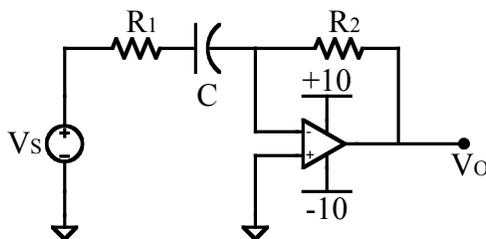
**Figure 8. An Active High Pass Filter.**
