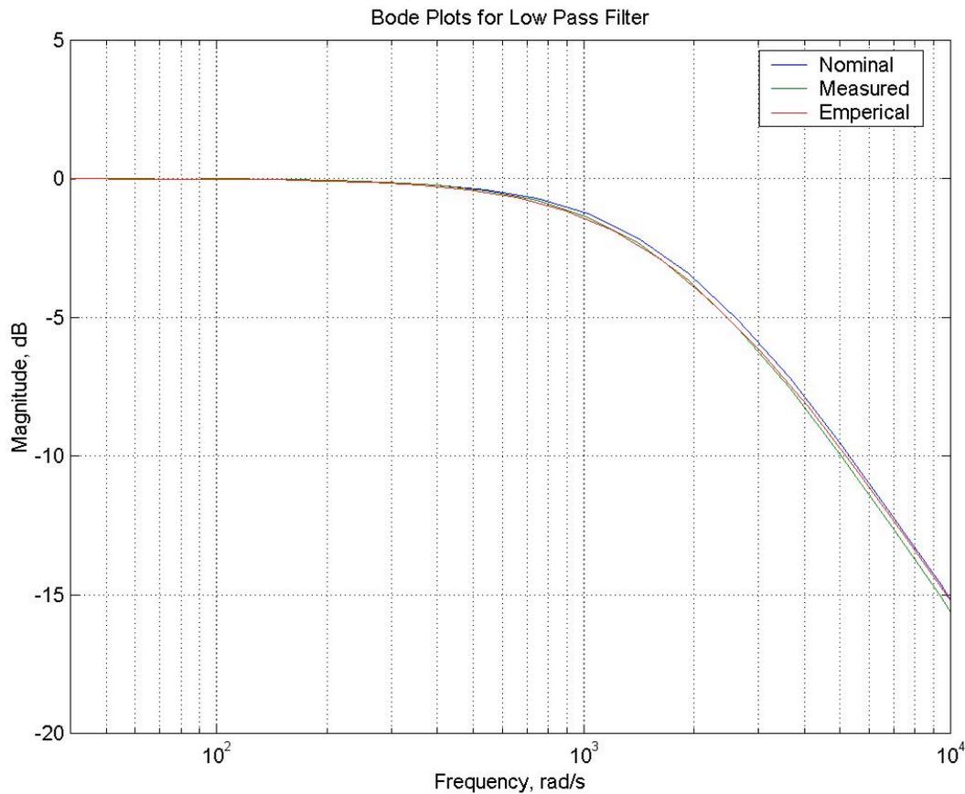
Figure 13. Example Bode Plots for a Low Pass Filter.
