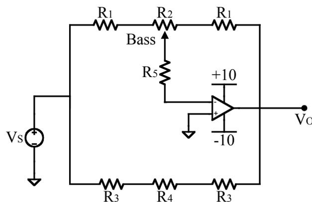
**Figure 11. Bass Controller at Low Frequencies.**
