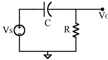
**Figure 4. An RC High Pass Filter.**
