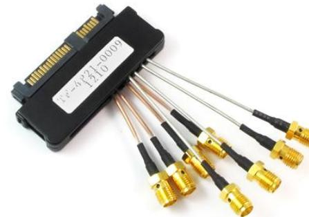
SAS Dual Port Receptacle Test Fixture
