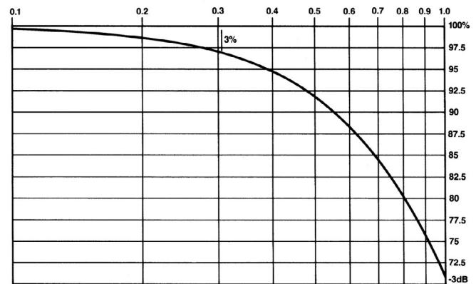
Figure 4.8. Bandwidth derating curve.
