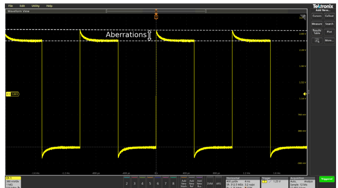
Figure 10.2. Aberrations from over-compensating a probe.
