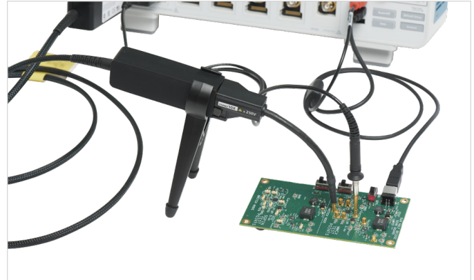
Figure 3.7. IsoVu optically isolated probes have high bandwidth and extremely high common mode rejection.
