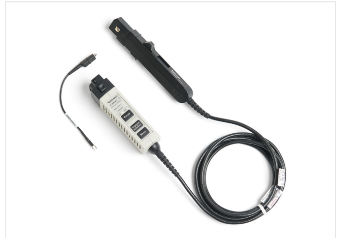
Figure 3.12. An example of a split core AC/DC current probe. It includes a split core transformer in the jaw as well as a hall sensor with supporting electronics for measuring DC current.
