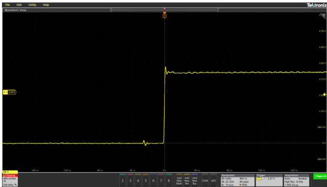
Figure 6.7. 1.5 ns rise time step waveform as acquired through a PCB to probe-tip adaptor.
