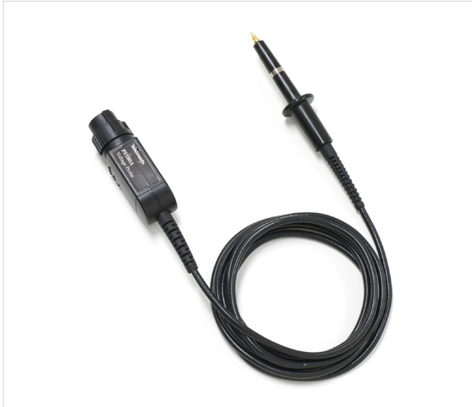
Figure 3.6. High-voltage probes can measure DC voltages up to 20 kV and pulses up to 40 kV with a bandwidth of 75 MHz.
