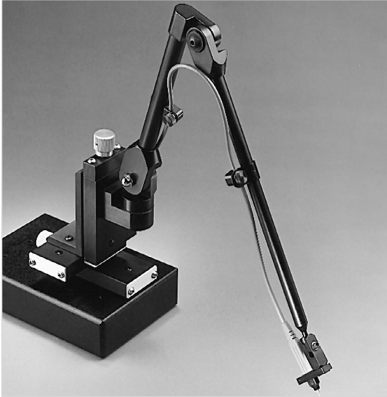
Figure 3.14. Example of a probing station designed for probing small geometry devices such as hybrid circuits and ICs.
