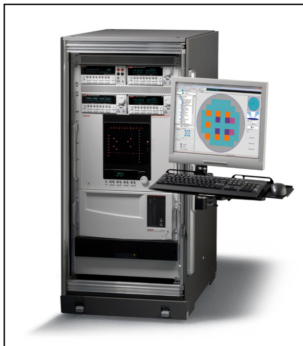
Figure 1. Example Model 4200-SCS running ACS and controlling a switch matrix.
