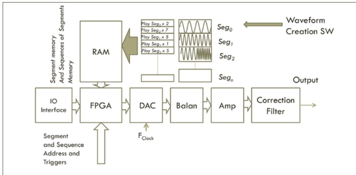
The Tektronix RFXpress® software is used to generate various RF waveforms that are loaded into the instrument through an I/O interface such as LAN, or PCIe. In some cases such as the Tektronix AWG70000 the waveform generation software is native to the instrument, in other cases a separate PC software program is used such as MATLAB®.
