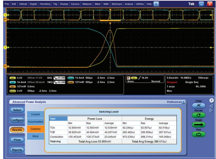
Figure 17. Automated measurement of switching loss using DPOPWR.
