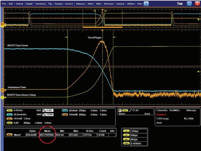
Figure 16. Switching loss measurement using oscilloscope's measurement toolset.
