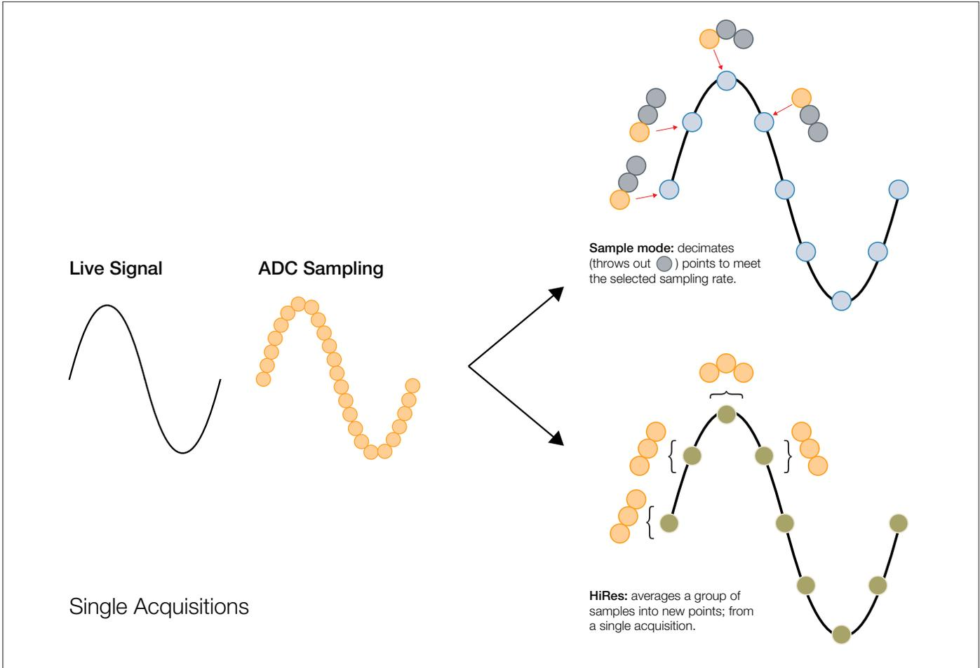
Figure 11. HiRes Acquisition Mode calculates the average of all the samples for each acquisition interval.
