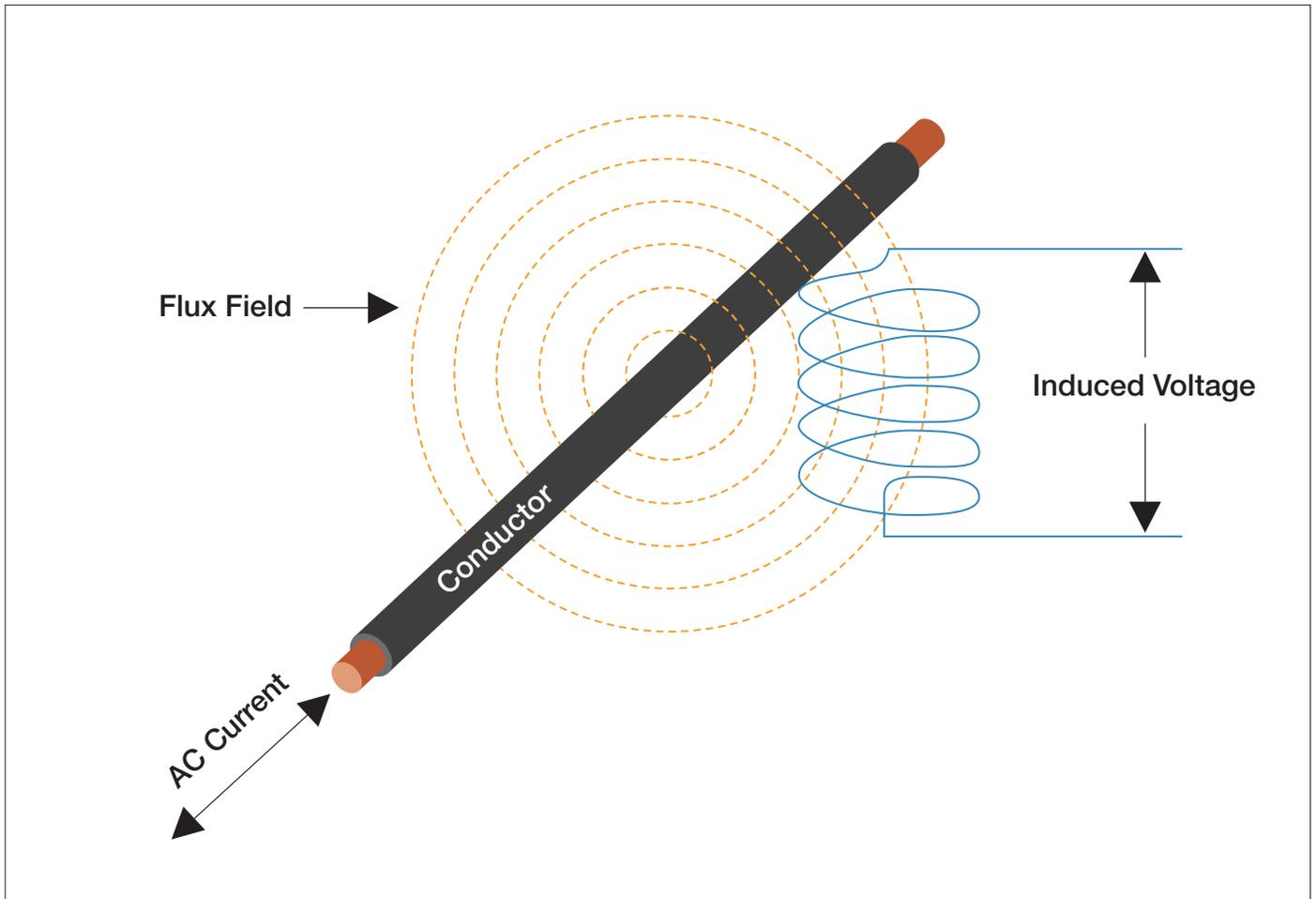
Figure 3. Alternating flux field induces voltage across a coupled coil.
