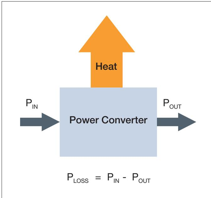
Figure 1. Loss due to power conversion inefficiency.
