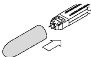
Protect the probe tips with the protective cover
