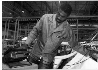
much more accurate, and it's easier for our people to use. In the past, with analog meters, it was necessary for us to zero out the instrument each time we used it. That's not required, of course, with the 580's digital readout.
