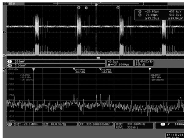
**MDO4000查找射频嵌入式系统电路板中的EMI**
