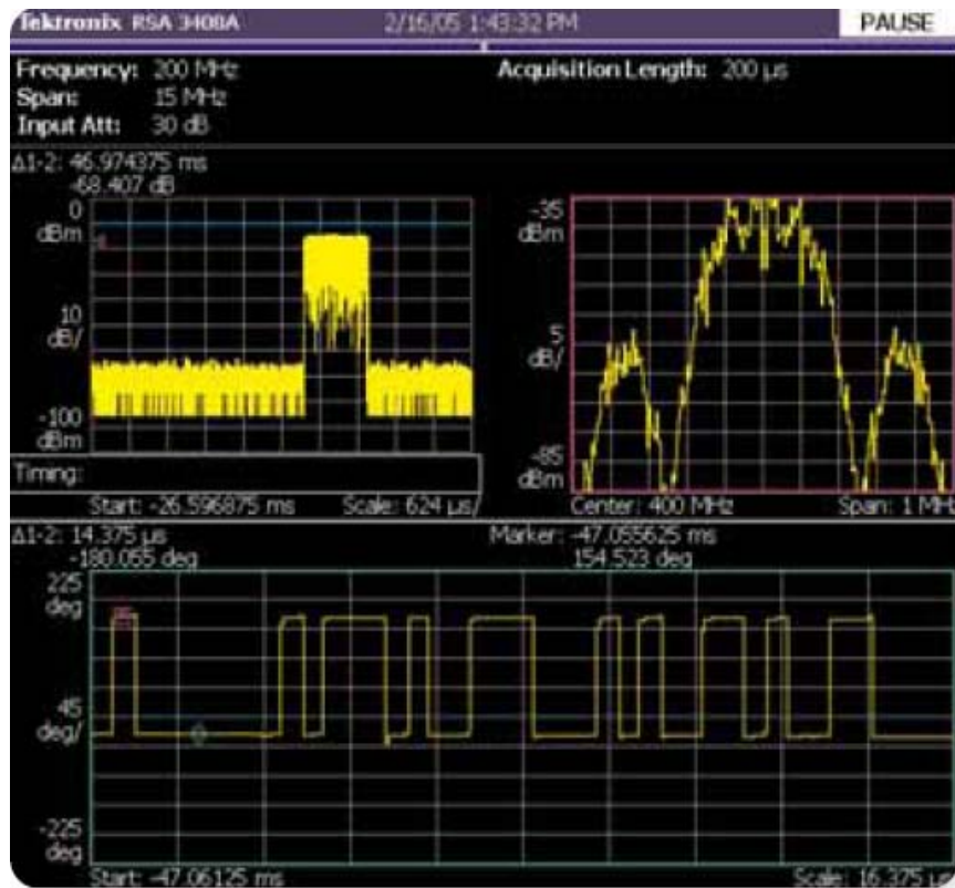
► Figure 27. 180° phase transitions are examined on a bi-phase modulated compressed pulse.
