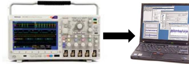
MATLAB acquires waveforms for custom measurement and analysis
