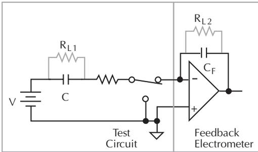
$$\text{Gain: } 1 + \frac{j\omega C + 1/R_{L1}}{j\omega C_F + 1/R_{L2}}$$
