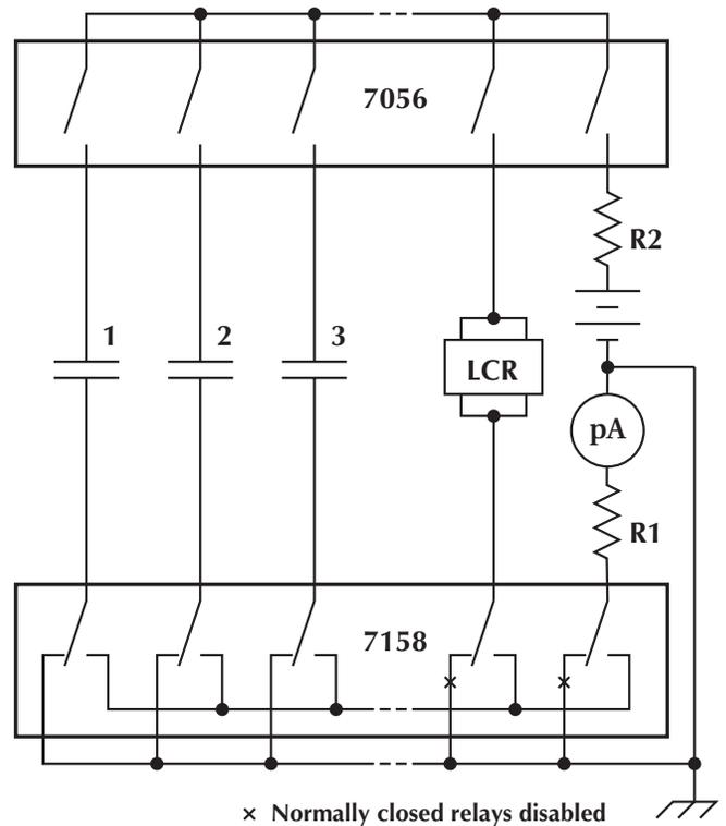
Figure 6. Capacitance and IR measurement system
