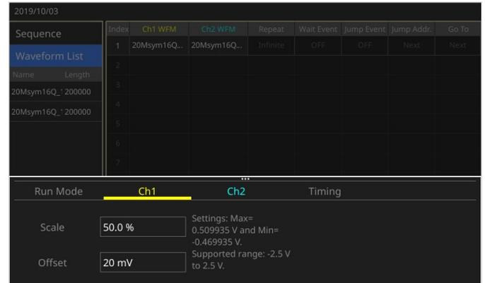
The final setting is the **sample rate** for the waveforms. Touch the **Timing** tab and set the sample rate to the same value that was noted from the Setup>Acquire tab in the RSA before the TIQ file was saved.
