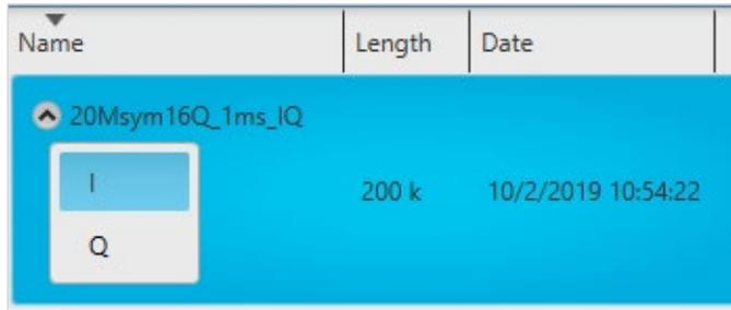
Right-click on the “I” waveform, and select **Save As...** In the Save As.. dialog box, navigate to where you want to save the waveform, enter the desired filename, change the “Save as type” selection to **AWG400/500/600/700 Waveform (\*.wfm)** type and then hit **Save**.
