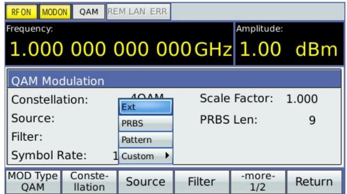
To create the output, simply hit the **RF** and **Mod ON/OFF** keys (translucent). They will illuminate when active.
