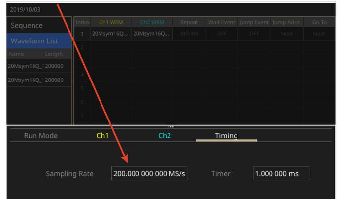
To run these waveforms, hit the Ch1 and Ch2 “On” keys, then hit the **Run** key on the front panel. Note that any changes in the Settings Bar menu will only take effect after toggling the **Run** key off and on again.
