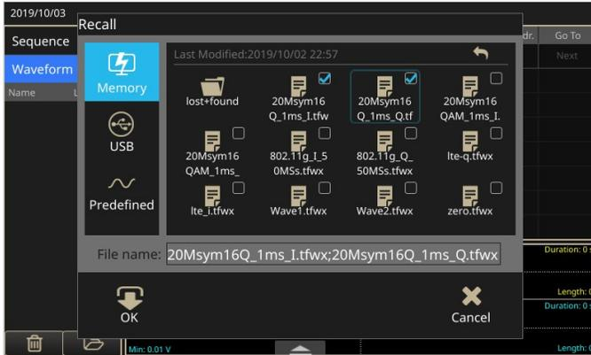
Touch the icons of the waveforms you wish to load into the waveform list (checkmarks will appear on those selected) and touch the **OK** icon. These waveforms will then be loaded into the waveform list.
