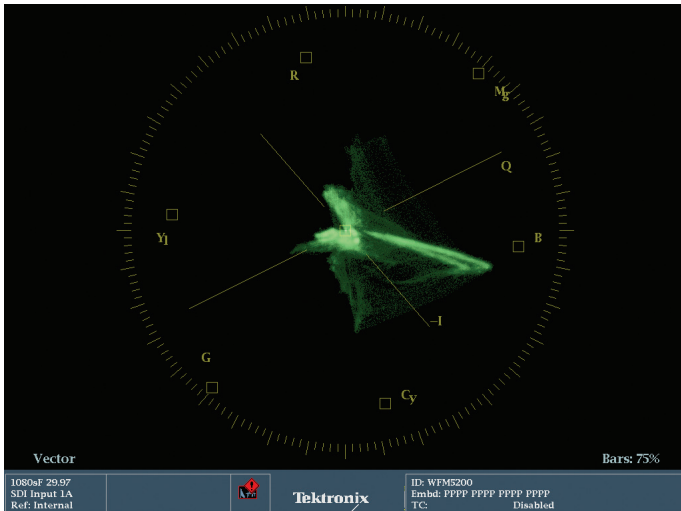
Figure 1-6. The graticule is the part colored gold and the trace is colored green. The colors of the graticule and trace are user selectable. These are the defaults. Many colorists prefer to use white or gray only to keep their eyes from being affected by the saturation of the colors.
