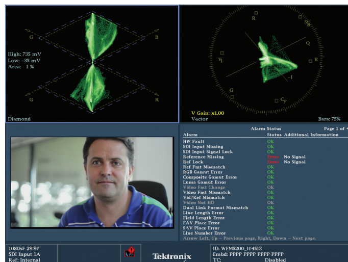
Figure 5-19. Four tile display with Tektronix Diamond display of uncorrected image.
