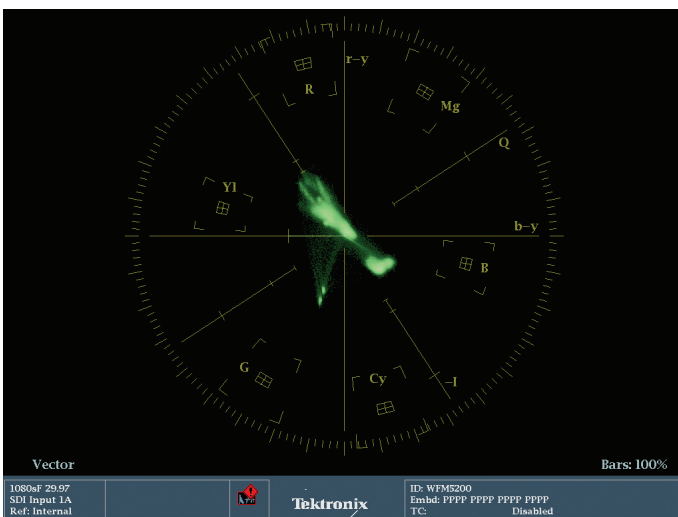
Figure 4-36. This is the vectorscope image representing the footage of the Marine with binoculars. Note the two small dots extending towards the green trace. These are the two green reflections on the lens of the binoculars. The trace showing the warm flesh and earth tones and the blue of the sky are also clearly visible.
