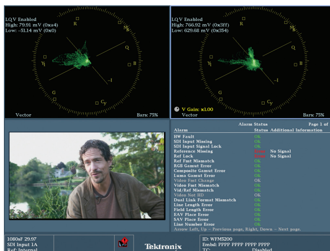
Figure 2-22. The HIGH and LOW Luma Qualified Vectorscopes are set up in the top two quadrants with the highlights on the shadows displayed on the left top quadrant and the shadows displayed on the right top quadrant.
