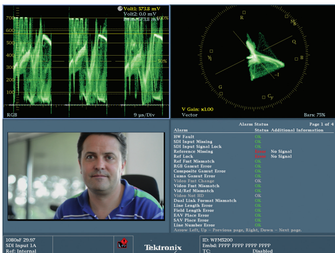
Figure 5-20. Our main camera with the “hero” grade. Note that the CURSOR was turned on and adjusted to better judge the relative color channel levels of the part of the trace indicating the gray wall behind the subject’s head.
