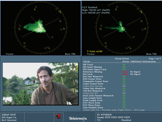
Figure 2-29. A third possible LQV display configuration with one LQV for highlights and one with a standard vectorscope.
