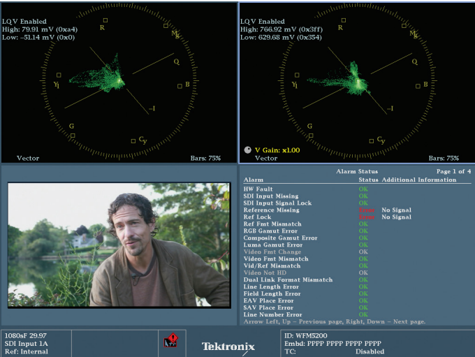
Figure 2-27. LQV Highlights and shadows. One possible LQV display configuration with one LQV for highlights and one LQV for shadows.
