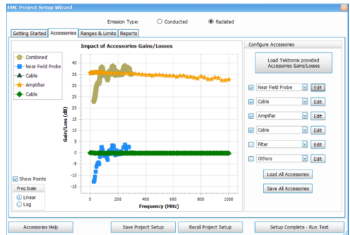
FIGURE 10. The combined impact is calculated only for the accessories common frequency range.
