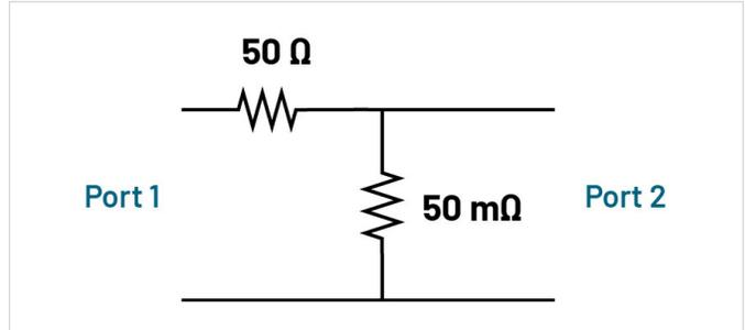
Figure 1. A simple shunt resistor circuit configured for an S21 measurement on a vector network analyzer (VNA).
