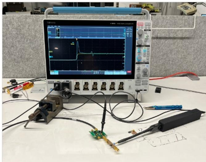
The current shunt probe being used in this example is a Tektronix TICP Series IsoVu Isolated Current Shunt Probe. To measure the signal off a shunt, a low-noise isolated probe like TICP is ideal. Isolation allows for the shunt to be placed anywhere in the circuit, even on a 1800 V voltage rail. And the low noise architecture provides a greater sensitivity than any high impedance probe. The probe faithfully measures the overshoot from the shunt in this example.
