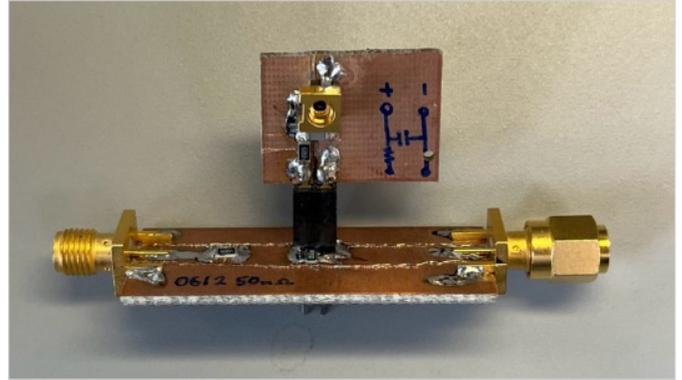
Figure 8. Shunt fixture with low-pass RC filter installed.
