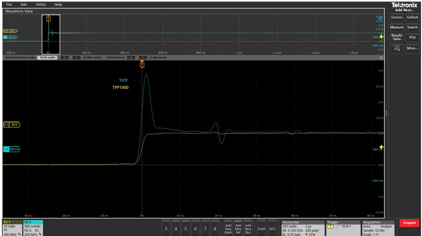
**Figure 4.** Measurements of edges from a fast step generator. The yellow trace is measured using a 1 GHz passive probe connected directly to the generator output. The blue trace is from a current shunt probe measuring across the 50 mΩ shunt resistor, which is connected to the same generator output.
