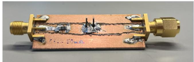
Figure 2. The circuit from Figure 1 with a 50 mΩ thin film shunt resistor, in an 0612 package mounted on a fixture. Port 2 is across the square pins tied to the shunt resistor in the center of the PCB.
