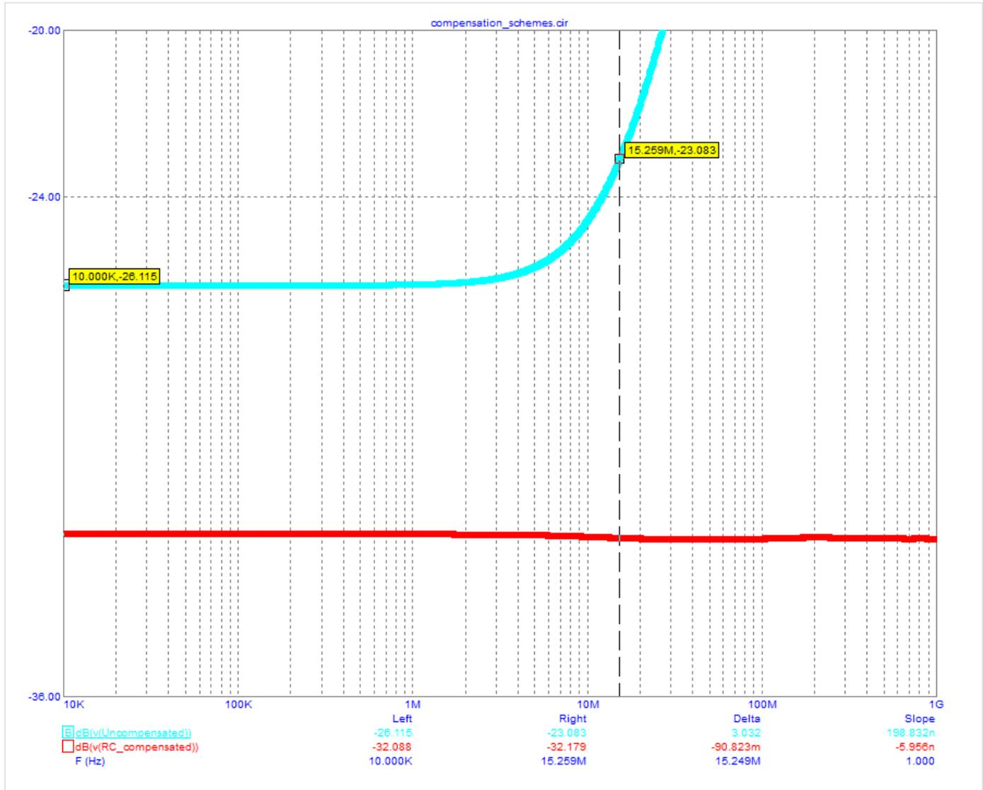
Figure 6. The upper, blue trace shows the response of the uncompensated shunt to an AC analysis, with a corner frequency of 15.3 MHz. The lower trace shows the much flatter response of the same circuit with an added RC filter.
