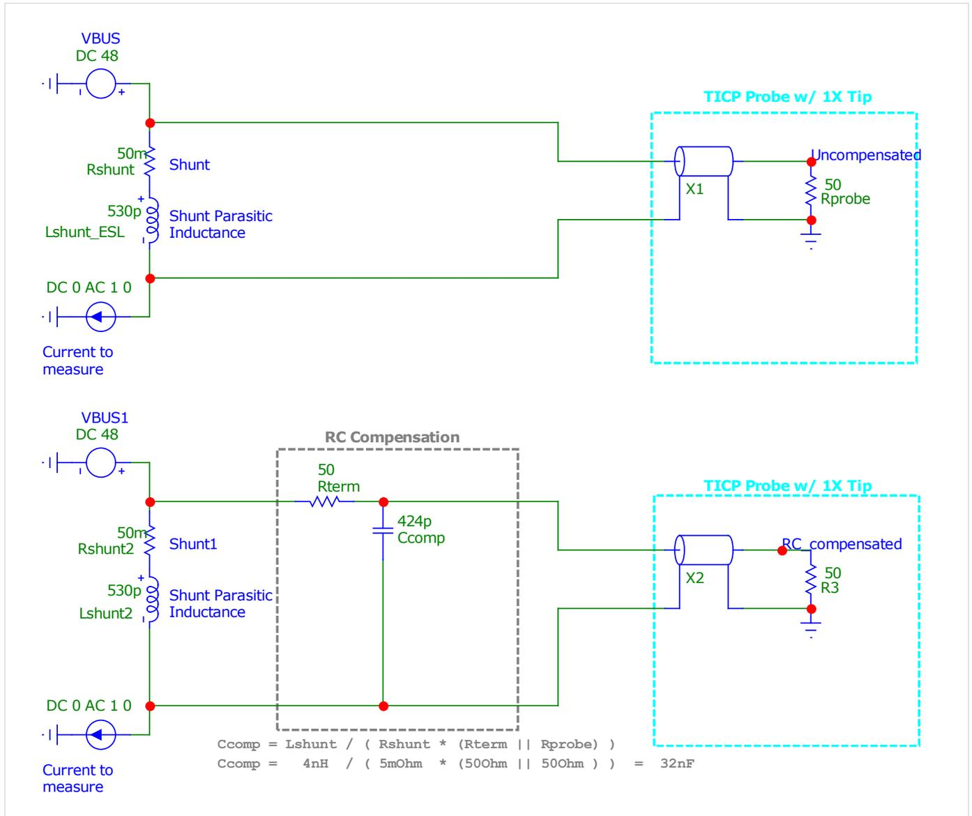
Figure 5. In the upper model iterative estimates of ESL are plugged in until the 15.1 MHz corner frequency is duplicated in the AC simulation. In the lower model, an RC filter with R=50 Ω is inserted into the circuit to counteract the parasitic inductance in the shunt. The results of these two simulations are shown in Figure 5.
