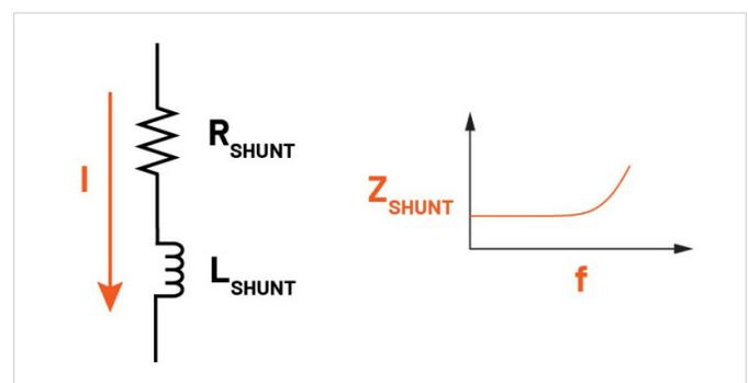
Figure 1. Especially with low-value shunt resistors, parasitic inductance will begin to impact the overall shunt impedance at frequencies above 1 MHz.
