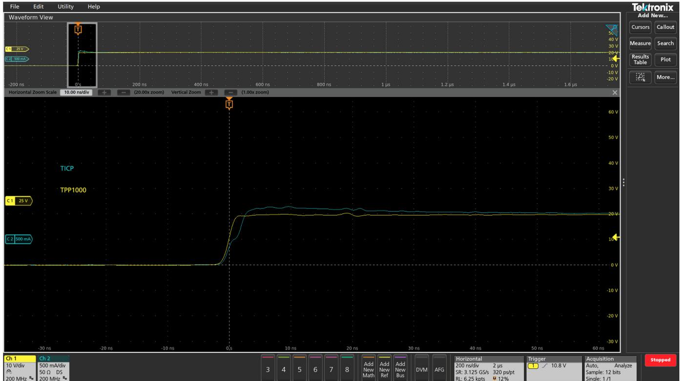
Figure 10. Measurements of edges from a fast step generator, similar to Figure 4 but with an low-pass RC filter applied across the shunt. The yellow trace is measured using a 1 GHz passive probe connected directly to the generator output. The blue trace is from a current shunt probe measuring across the 50 mΩ shunt with a low-pass filter installed (R=50 Ω and C=547 pF).
