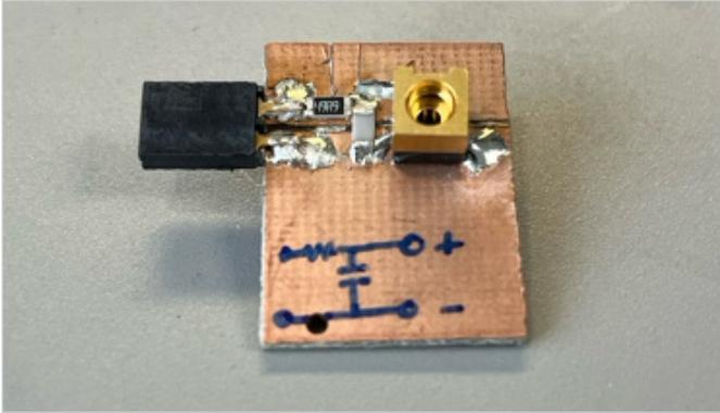
Figure 7. A low-pass RC filter, with  $R=50\ \Omega$  and  $C=547\ \text{pF}$ , based on the results of simulations.
