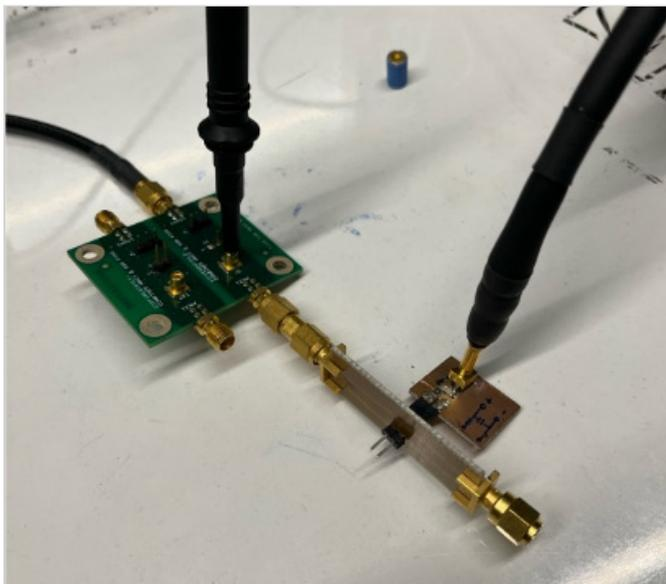
Further improvements are possible with multi-pole designs and more accurate modeling of shunt behavior. As you may expect, the filter boards themselves have their own parasitic elements that also must be compensated, in an infinite loop of diminishing returns. The parasitic elements can be seen in the VNA data above 280 MHz where the shunt plus filter response returns to being strongly inductive.
