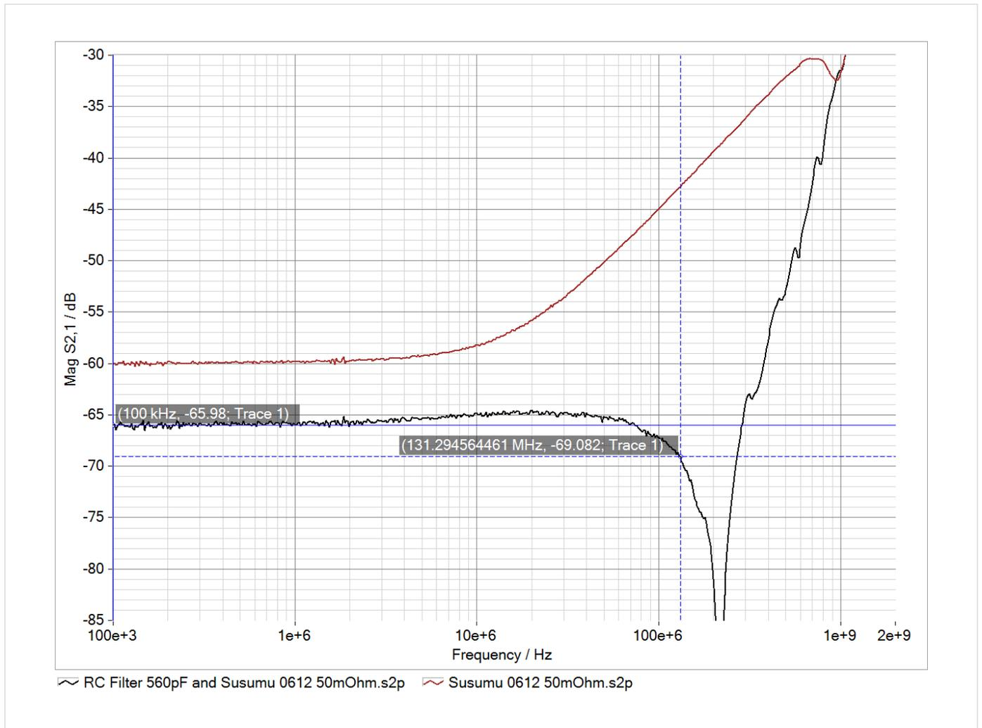
Figure 9. The upper (red) trace represents the frequency response of the uncompensated shunt resistor. The lower (black) trace represents the frequency response of the combined network with RC compensation.
