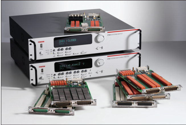
Figure 3. The Model 3740 32-Channel Isolated Switch Card is part of the Series 3700 Switch System/Multimeter family. The system's mainframe contains six slots for plug-in cards in a compact 2U high (3.5 inches/89mm) enclosure that easily accommodates the needs of medium to high channel count applications. A fully loaded mainframe can support up to 576 two-wire multiplexer channels.
