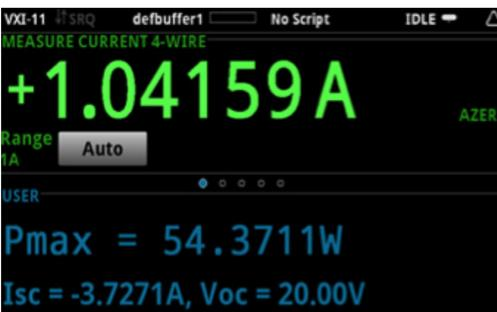
**5** Some instruments can directly display power and solar cell max power, short circuit current, and open circuit voltage.
