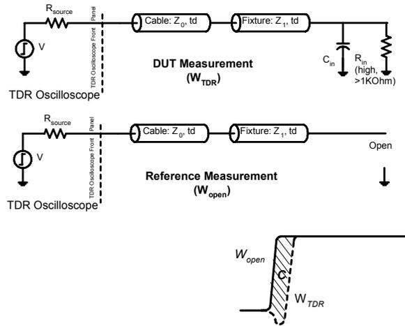
**Figure 2. Self-capacitance measurement.**
