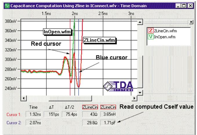
**Figure 8. Reading the capacitance value from the true impedance profile computed in IConnect. Note the placement of cursors.**
