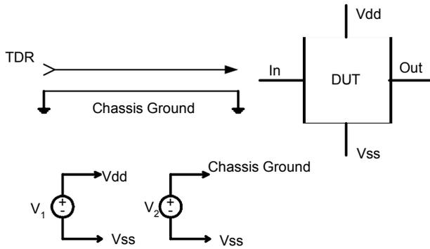
**Figure 5. Measurement set up of chassis ground in reference to DUT ground. Since the power supplies float relative to the chassis ground, changing  $V_2$  allows us to vary the TDR offset voltage to DUT  $V_{ss}$ .**
