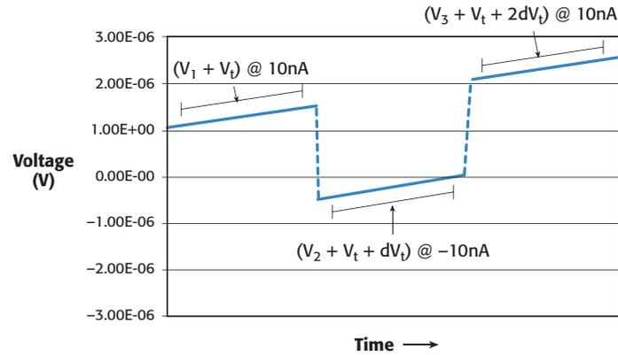
$$V_a = \text{negative-going step} = \frac{(V_1 + V_t) - (V_2 + V_t + dV_t)}{2} = \frac{(V_1 - V_2 - dV_t)}{2}$$
