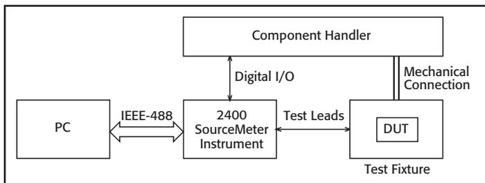
Figure 2. 2400-Based Resistor Production Test System..
