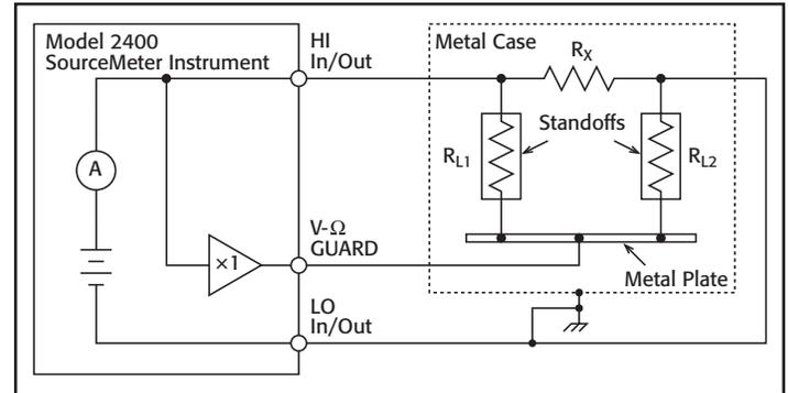
Figure 5. Model 2400's Built-In Guard.
