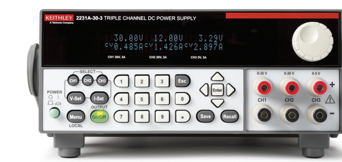
Low-Voltage DC Supply - Powers Gate Drive Electronics
