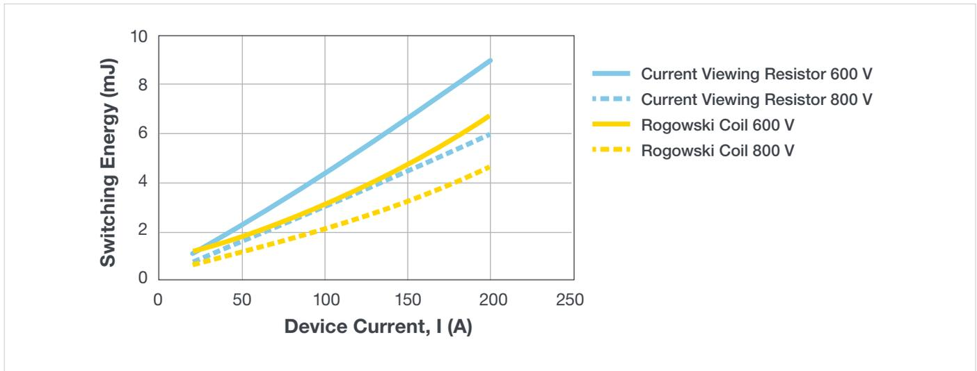
Figure 10. Switching loss ( $E_{off} + E_{on}$ ) estimation using different probes (CAB011M12FM3,  $T_J = 150\text{ }^\circ\text{C}$ ,  $R_G = 1\ \Omega$ ).
