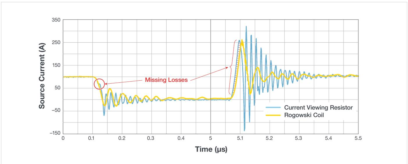
Figure 9. CVR vs Rogowski Current Probe, CAB011M12FM3 (T<sub>J</sub> = 150°C, R<sub>G</sub> = 1 Ω, V<sub>DS</sub> = 600 V, I<sub>S</sub> = 100 A).
