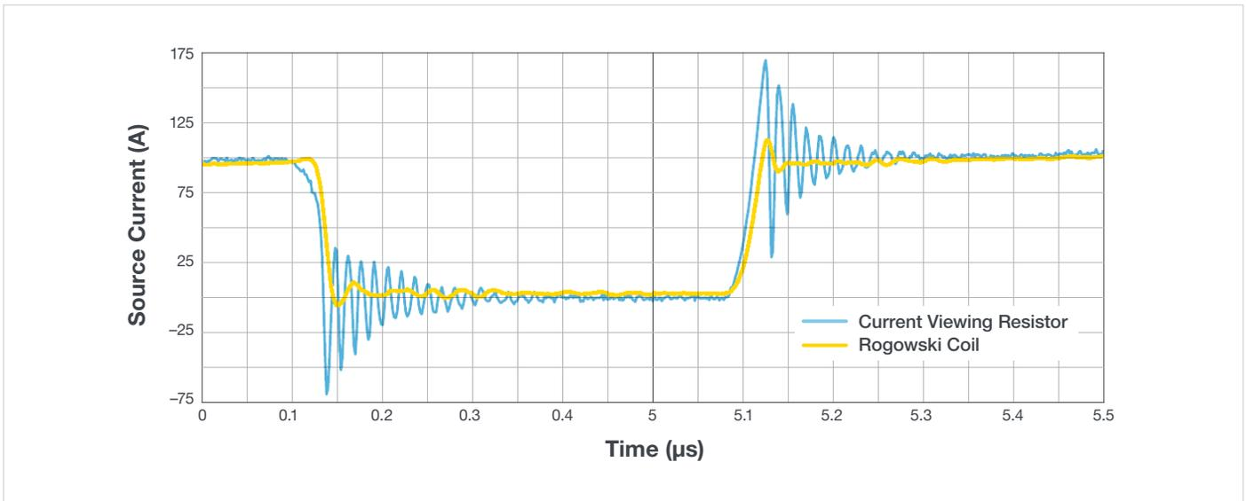
Figure 8. CVR vs Rogowski Current Probe, CAB016M12FM3 (T<sub>J</sub> = 25°C, R<sub>G</sub> = 6.8, V<sub>os</sub> = 600 V, I<sub>s</sub> = 100 A).
