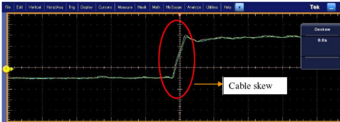
Figure 36. Visible Cable De-skew
