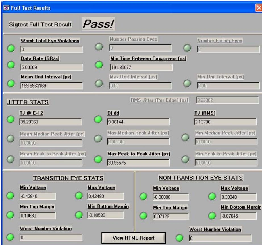
Figure 26. SIGTEST Jitter Results
