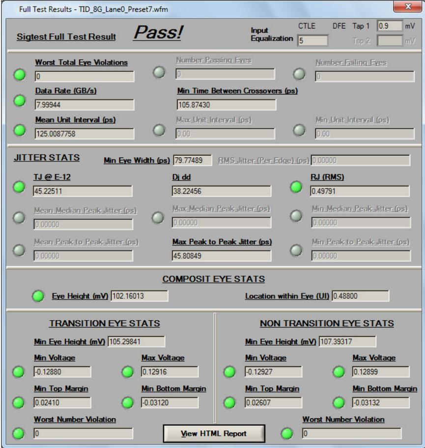
Figure 28. SIGTEST Jitter Results
