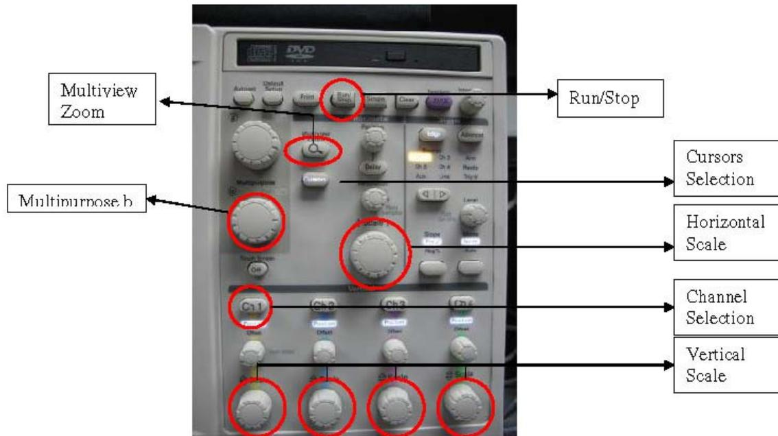
**Figure 20. MSO/DSA72004 Scope Front Panel**
