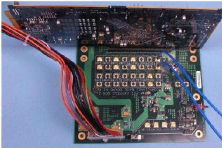
Figure 9. CBB lane 0 connected to SMP end of cables
