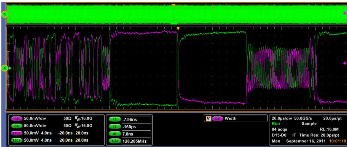
Figure 19. Single Ended Data scale adjusted to full scale without any clipping Gen 3
