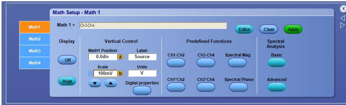
Figure 11. Math Function set-up to get differential signal (MSO/DSA72004 Scope)
