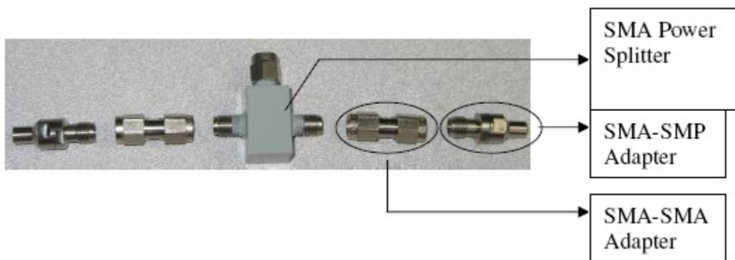
Figure 3. Miscellaneous components required for cable de-skew etc
