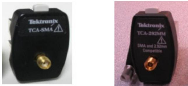
Figure 4. TCA-SMA Adapter and TCA-292MM Adapter
