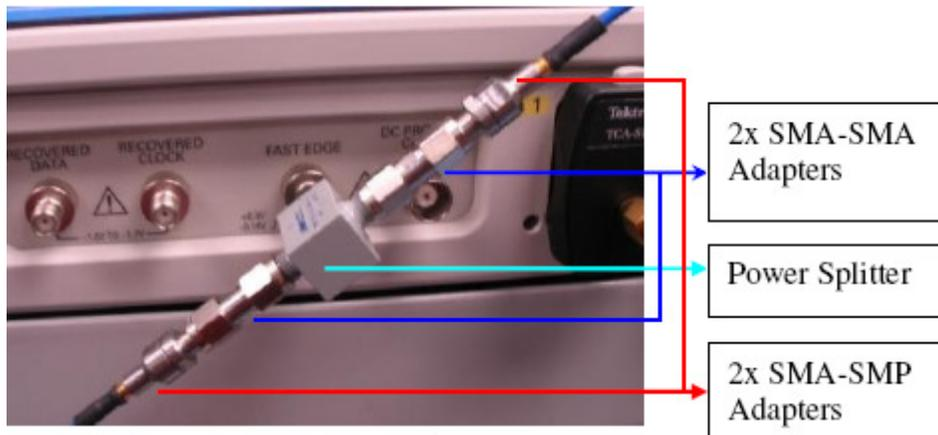
**Figure 34. Cable de-skew connections**
