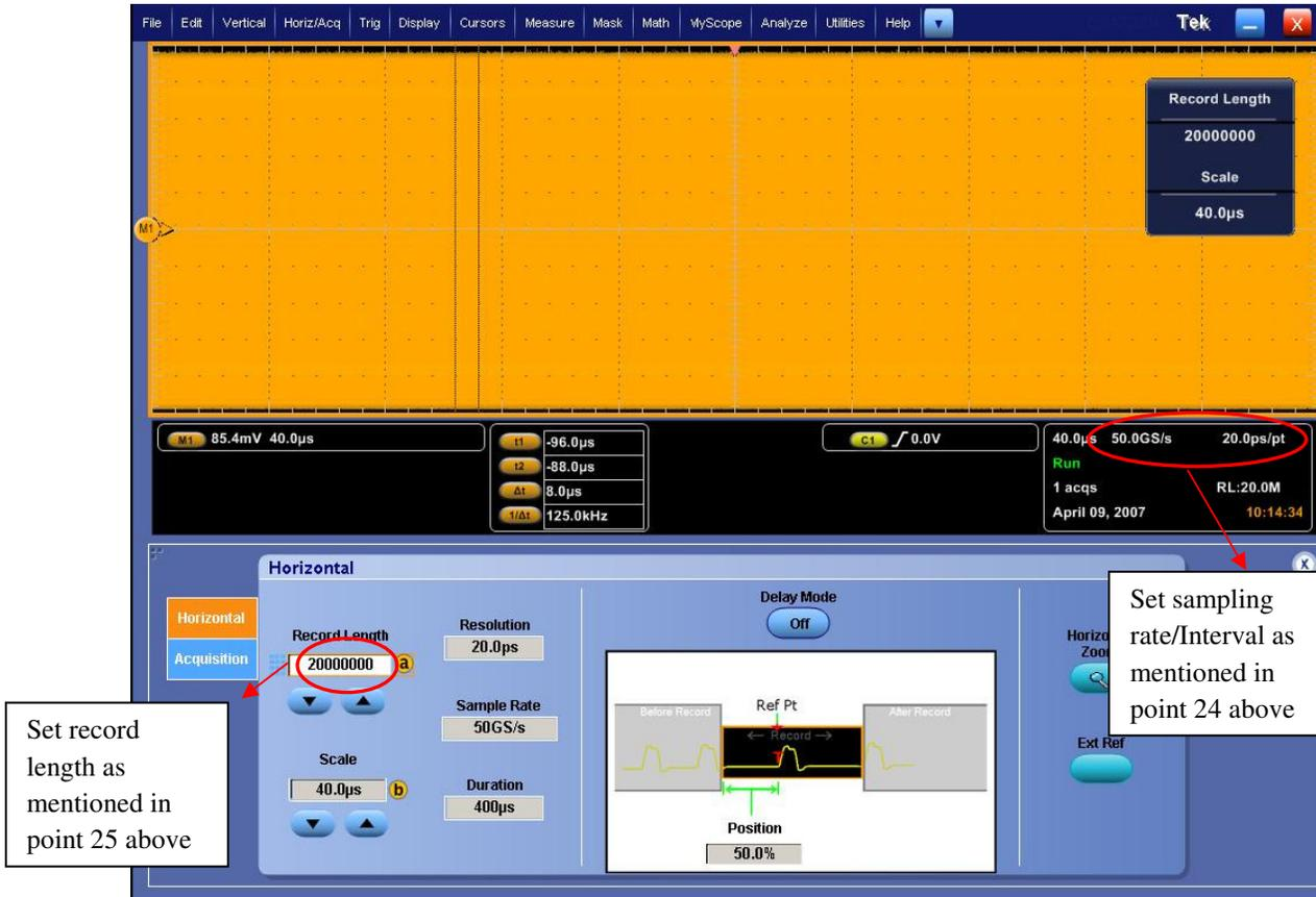
**Figure 14. Scope settings for waveform capture**
