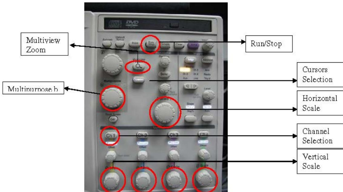
Figure 12. MSO/DSA72004 Scope Front Panel
