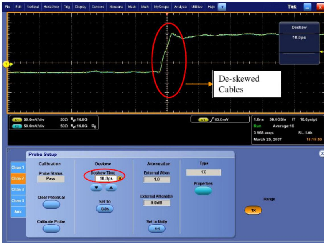
Figure 37. Cable Skew Adjusted
