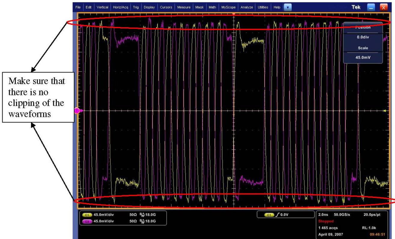
Figure 10. Single Ended Data full scale without clipping
