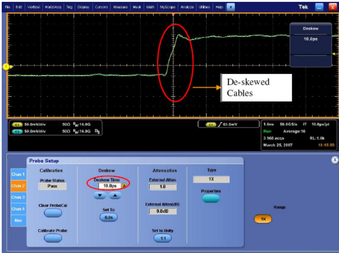
Figure 38. Cable Skew Adjusted
