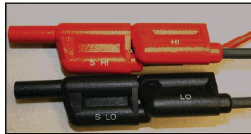
The jacks used on the test fixture should be high quality. In particular, some red jacks use high amounts of ferrous (Fe, iron) content to produce the red coloring, and these jacks can have unacceptably high levels of leakage due to conduction. The resistance between the plugs to the case should be as high as possible and in all cases  $>10^{10}\Omega$ .
