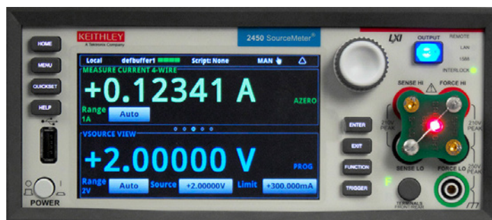
Figure 1. Model 2450 SourceMeter SMU Instrument measuring the I-V characteristics of a red LED.
